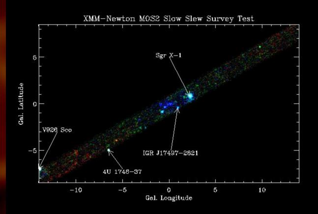
Slew rate: 30"/s Texp: 42,700s Effective: 40s (pn) Overlap: 15' Area: 43°x2° b = +/-9° l = +/-15°Pos accuracy: < 4" Flim (soft): 2.0 10<sup>-13</sup> erg/s/cm<sup>2</sup> Flim (hard): 1.3 10<sup>-12</sup> erg/s/cm<sup>2</sup>
