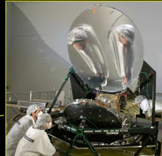
Planck Telescope 1.5x1.9m off-axis Gregorian T = 50 K
