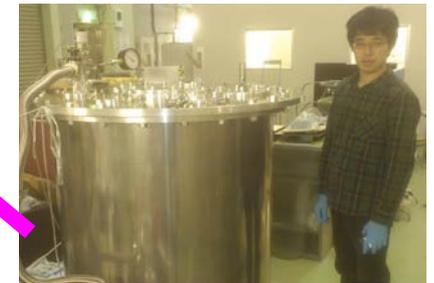
Cryostat cooled by PTC + Helium sorption cooler
