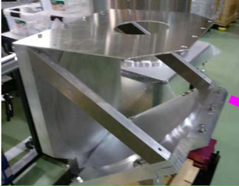
**Cold optics** at 4 K, Mizuguchi-Dragone dual-reflector, 20° FoV, angular resolution of 0.6° at 145 GHz
