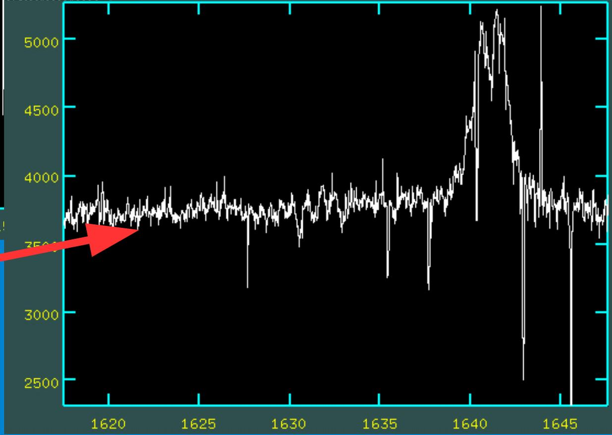
MODAL NOISE (fibres!) degrades signal-to-noise
