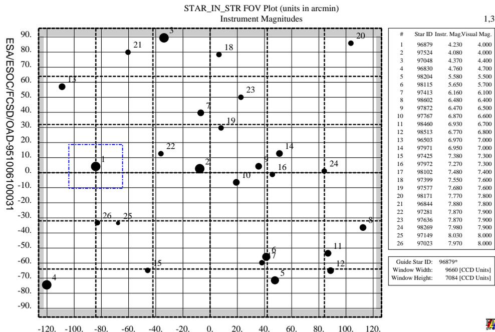
Figure 2. A typical star tracker field of view taken from the ISO mission. The restricted search window can be seen in the left half of the field of view. The XMM and INTEGRAL missions will make use of a similar star tracker design.
