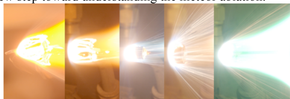
Fig 1 Meteor ablation by arc-heated wind tunnel. 2 Meteorites (left) and 3 artificial meteor samples (right).
