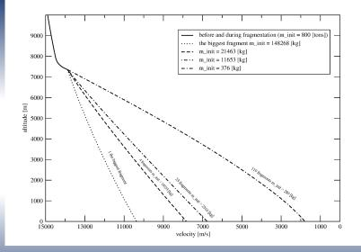
$m_{init} = 800 \ [tons] \ \theta_{init} = 40 \ [^{\circ}] \ v_{init} = 16 \ [km/s]$
