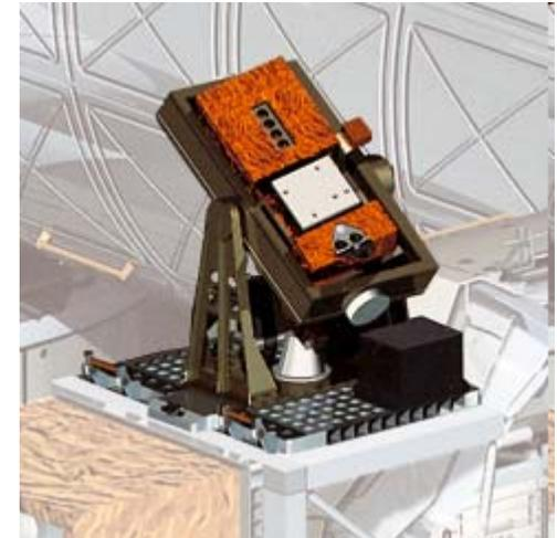
SOLAR is a set of three instruments monitoring solar output.
