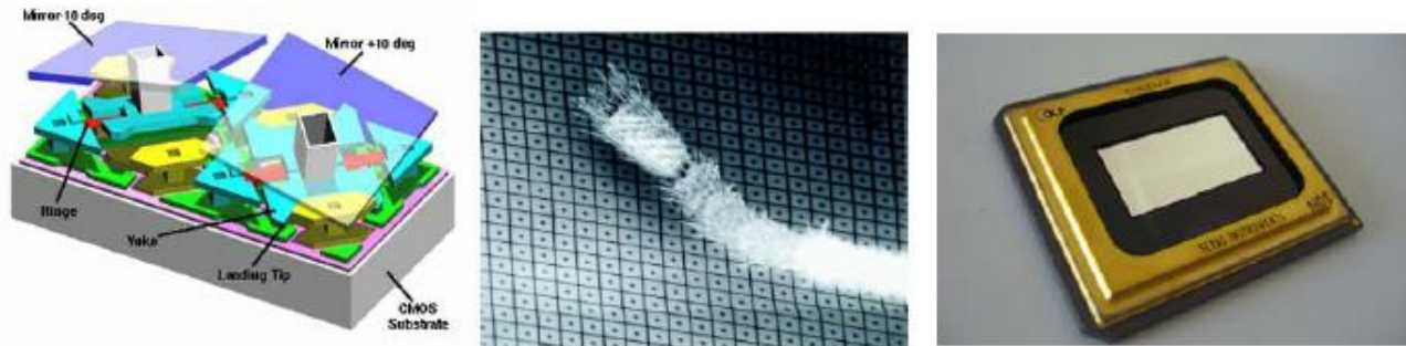
Fig. 1. Typical substructure of a TI DMD (left); DMD array with an ant leg for comparison (centre); DMD CINEMA (right).
