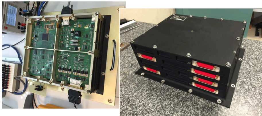
Figure 10: Two views of the EM PMCU which controls the shutter, calibration unit and provides the thermal control of the FPA.
