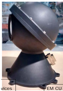
Figure 8: The EM Calibration Unit. This unit lacks the baffle on the exit port (on the left) with its field stop and lens system.
