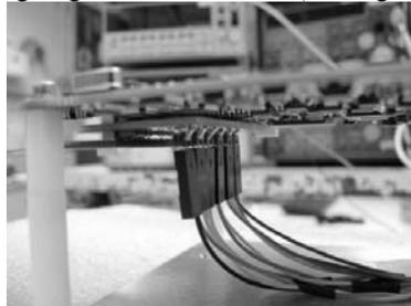
Figure 11 PCB board allowing power consumption measurement situated between the JADE2 card and the flex cable to the SIDECAR
