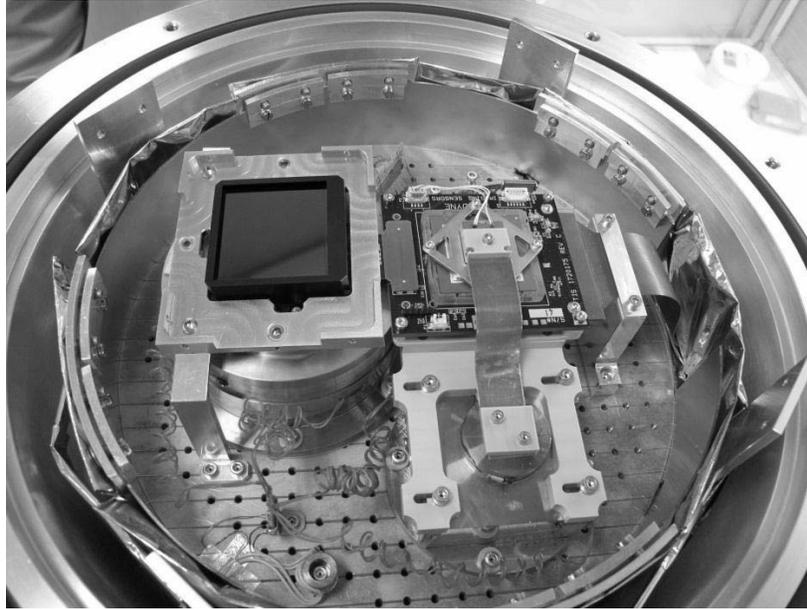
Figure 2 Overview of the system HAWAII-2RG SIDECAR ASIC
