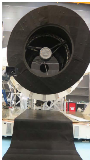
Figure 8. Front view of the telescope & baffle with the black blankets set-up for the straylight test(Courtesy Airbus Defense&Space).
