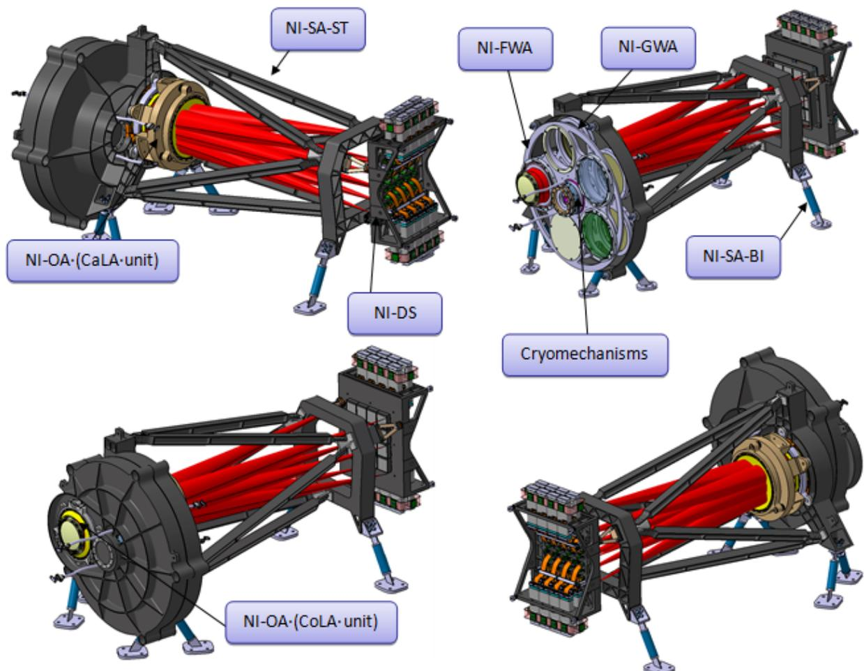
Figure 4-1: 4 views of the NI-OMA with the NI-DS mounted on it.
