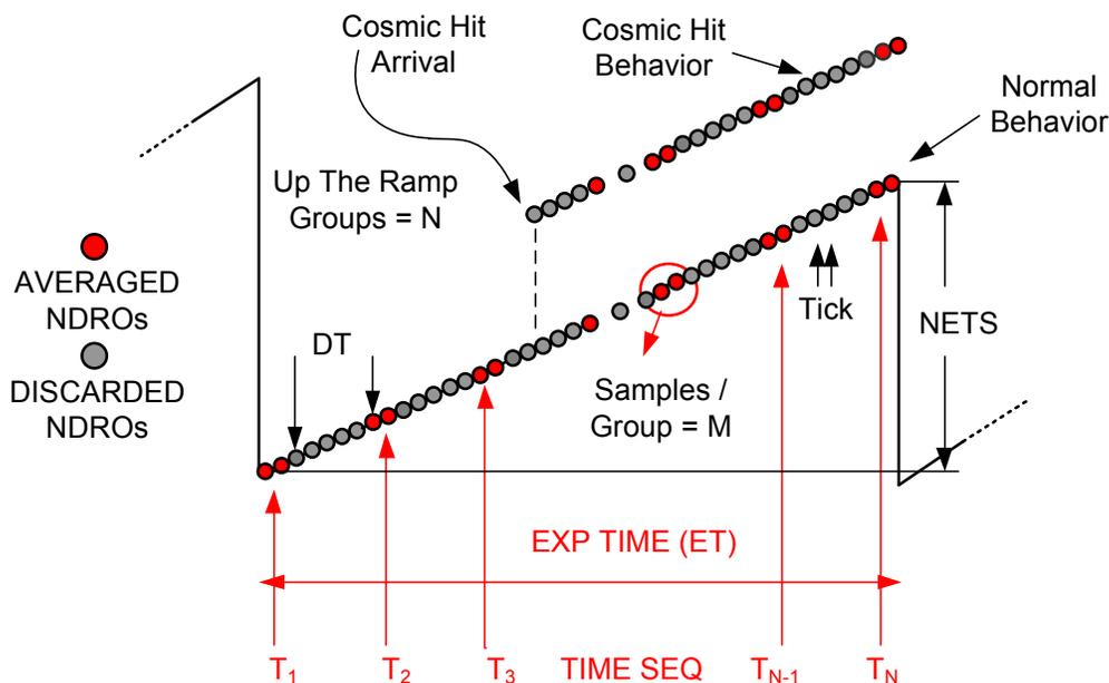
Figure 7-1: Scheme of the Multi Accumulation readout mode
