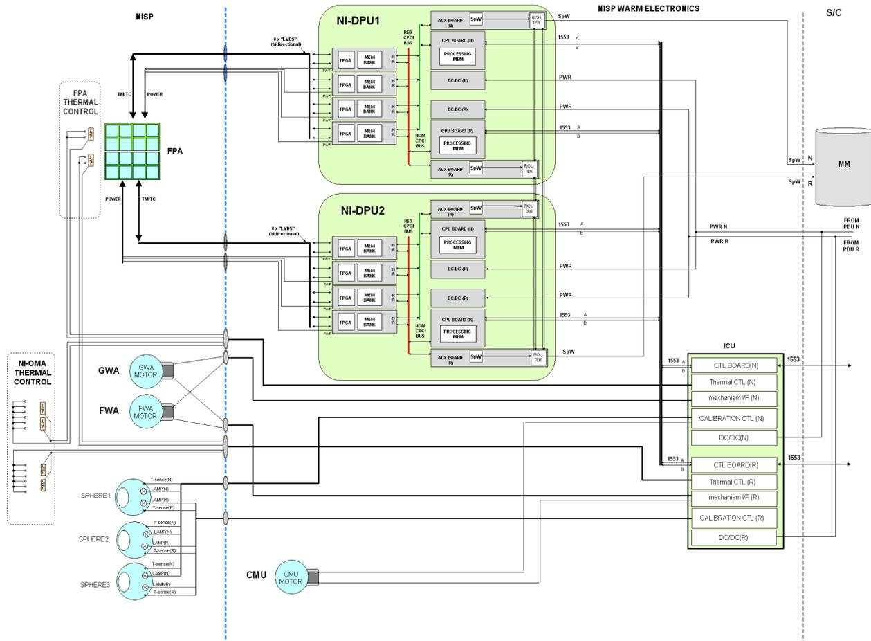
Figure 6-1: NISP Warm Electronic schematic view
