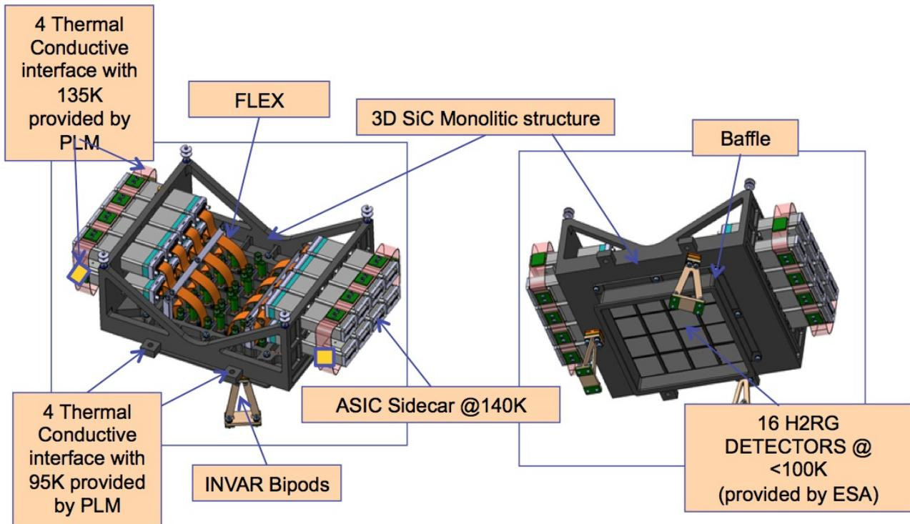
Figure 5-2: The NISP Detector System (NI-DS)
