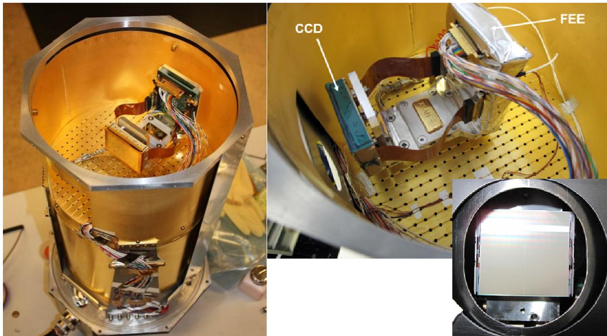
Figure 1: The CCD cryostat with vacuum enclosure removed (upside down). The plate with the regular grid of threaded holes is the bottom of the liquid nitrogen reservoir and acts as the sample stage for the CCD. The cylindrical enclosure is a 77K thermal shield, with an aperture for radiation access on the left hand side. The inset shows a Euclid prototype FI CCD273-84 as seen through the radiation access port of the cryostat.
