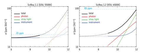
1-sigma photometric precision (in parts per million) for two sizing cases. Left: precision foreseen after a total on-source integration time of 6 hours (duration of transit of planet with orbital period of 50 days). **Right:** precision foreseen after a total on-source integration time of 3 hours (duration of transit of planet with orbital period of 13 days). The dashed horizontal lines denote requirements.
