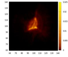
Left: White light PSF measured over 500 - 800 nm waveband during the on-ground calibration campaign (x- and y-axes in pixels relative to bottom lower left pixel in a 200x200 pixel image frame, colour scale indicates fraction of total power in an individual pixel); **Right:** Cuts through the PSF at the specified value of x. Credit: University of Bern.
