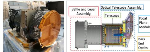
Left: Fully-assembled flight model of the CHEOPS payload; Right: Cross-section through the pavload. Credit: University of Bern.
