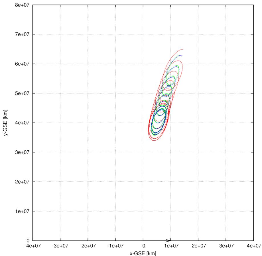
**Figure 2: Example constellation dynamics in the Geocentric Solar Ecliptic frame. The Earth is at [0,0]. The constellation starts close to the Earth (18 degree initial trailing angle) and then slowly moves away has been propagated for up to 10 years.**
