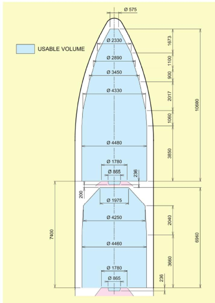
**Figure 5: A6 dual launch configuration with SYLDA under long fairing option. The SYLDA adapter has a mass of approx. 500 kg.**
