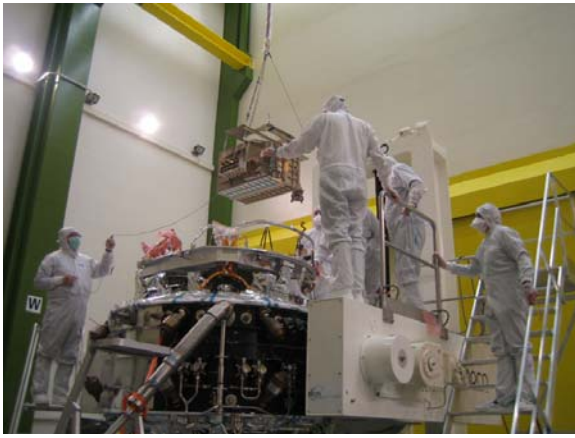
Figure 3. Two images of Herschel flight instrument integration onto the optical bench in Astrium, Friedrichshafen. On left SPIRE is being lifted, on the right all three focal plane units in place; on left HIFI, on right SPIRE, and in the background PACS. Images courtesy Astrium.
