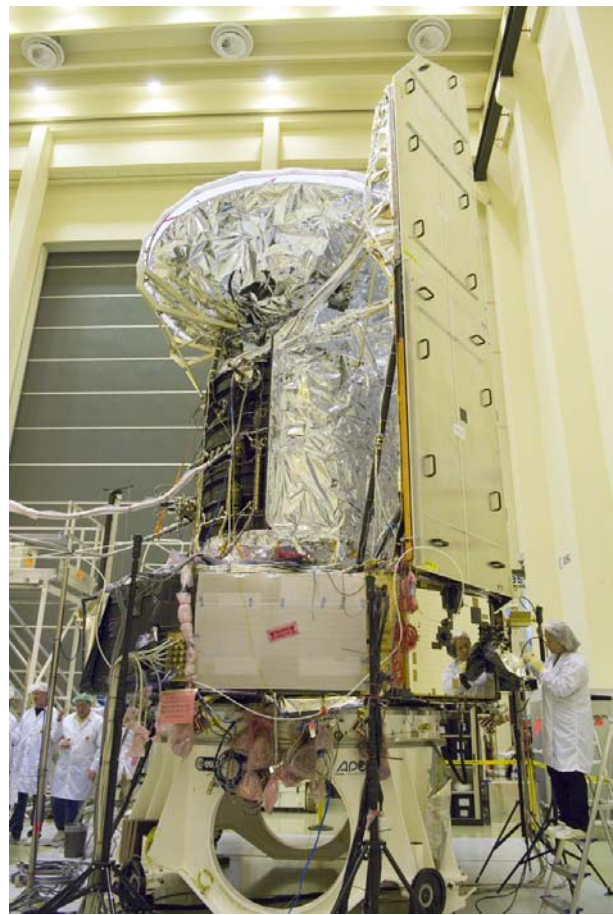
Figure 1. Two images of the Herschel spacecraft in the cleanroom in the ESTEC Test Centre. These pictures were taken on 23 April 2008 at the time when the spacecraft was very close to being mechanically completed in flight configuration. On the left a view of the side facing away from the sun. In the centre the black outside of the cryostat vacuum vessel (CVV) which will always be facing cold space inflight, below it the service module (SVM), and on the top of it the telescope protected by a cover which has its own support structure. Behind the spacecraft the backside of the solar array/sunshade (HSS) which is covered in multilayer insulation (MLI) to minimise thermal coupling. On the right a 'sideways' view, showing that the side of the CVV facing the HSS is also covered in MLI. The 'working' (sunward) side of the HSS is covered by protective elements, the handles for attaching and removing them are clearly visible. Images ESA.
