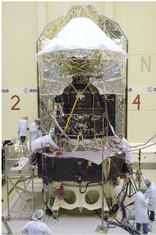
Figure 1. Two images of the Herschel spacecraft in the cleanroom in the ESTEC Test Centre. These pictures were taken on 23 April 2008 at the time when the spacecraft was very close to being mechanically completed in flight configuration. On the left a view of the side facing away from the sun. In the centre the black outside of the cryostat vacuum vessel (CVV) which will always be facing cold space inflight, below it the service module (SVM), and on the top of it the telescope protected by a cover which has its own support structure. Behind the spacecraft the backside of the solar array/sunshade (HSS) which is covered in multilayer insulation (MLI) to minimise thermal coupling. On the right a 'sideways' view, showing that the side of the CVV facing the HSS is also covered in MLI. The 'working' (sunward) side of the HSS is covered by protective elements, the handles for attaching and removing them are clearly visible. Images ESA.
