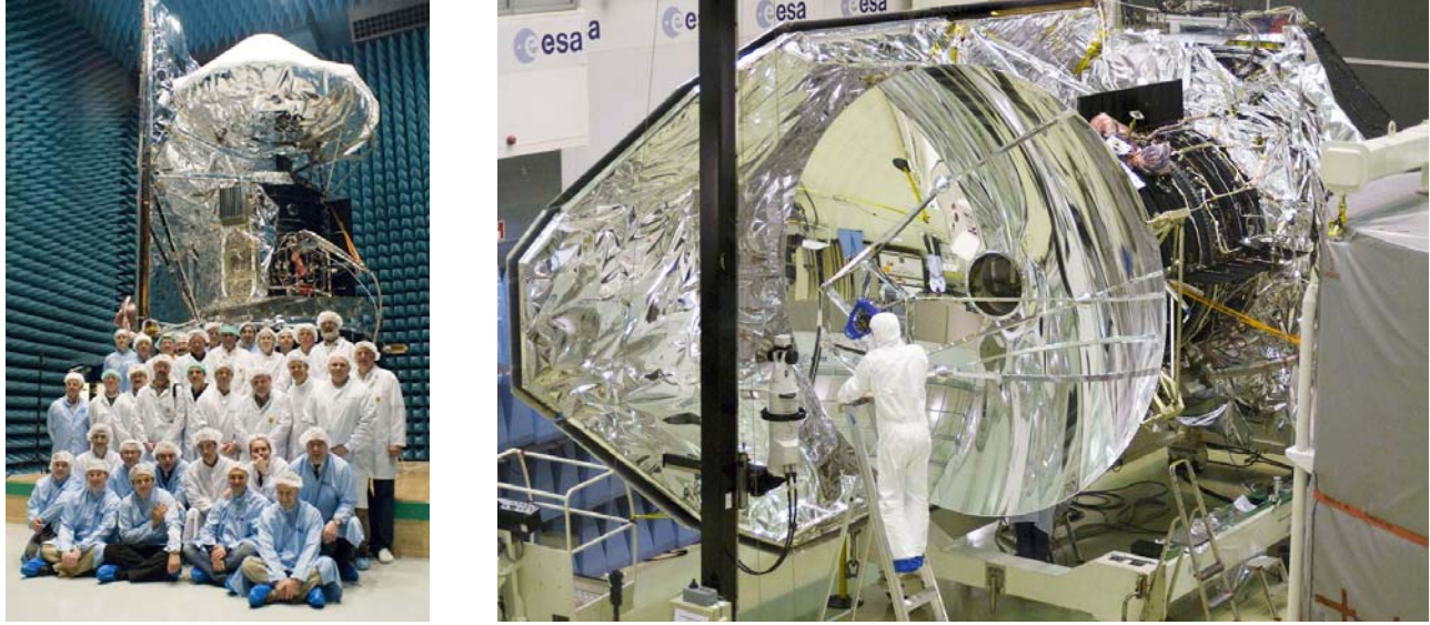
Figure 6. Herschel testing in the ESTEC Test Centre in May 2008. On the left Herschel in the Maxwell EMC chamber after conclusion of the testing with part of the industry and ESA team, on the right Herschel in a unique horizontal position for SPIRE spectrometer testing and M1-M2 reference measurements before spacecraft mechanical (vibration/acoustics) qualification. Images ESA.
