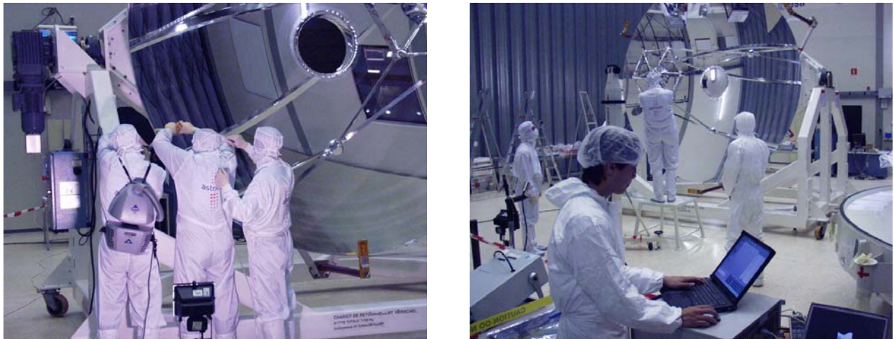
Figure 2. Two images of the Herschel telescope in the cleanroom in the ESTEC Test Centre. These pictures were taken shortly after unpacking during incoming inspection activities in late Jan 2008. In the left picture localised particulate contamination from the transport is removed, in the right picture preparations for a M1-M2 measurement are performed. Images ESA.
