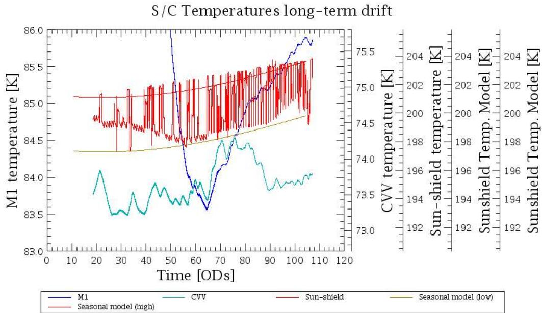
Figure 5: M1, CVV and sun-shield temperature variations since the start of the mission (CoP and PV phases together) compared to a sinusoidal model of the orbital evolution of the S/C temperature, with a minimum at the aphelion (on OD 22, July 4<sup>th</sup> 209) and a maximum on the perihelion (OD 204, January 4<sup>th</sup> 2010). The best fit model values to reproduce the sun-shield temperature trend have an amplitude of 2.3 K and a time-scale of half a year.
