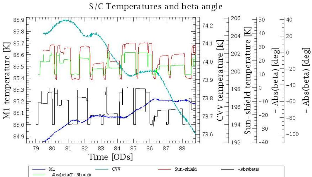
Figure 3: Zoom of Figure 2 showing the detailed match between the sun-shield temperatures and the inverse of the absolute value of the inclination angle beta. The measured time-delay between both curves is of 3 hours
