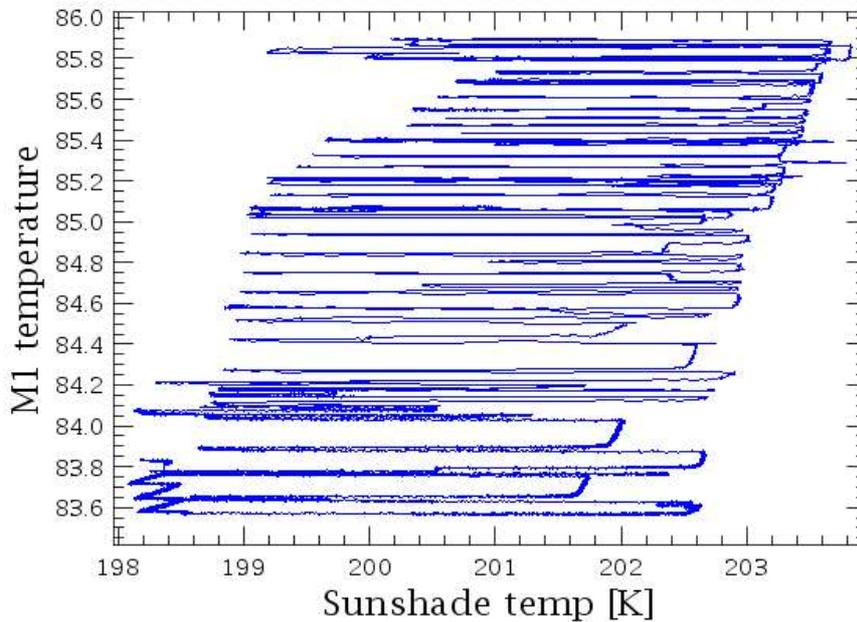
Figure 6: M1 temperature versus the sun-shield temperature from OD 70 to 100. In spite of the large 3-4 K departures of the sun-shield temperatures, an overall mirror temperature increase of 2.2 K can be measured over a mean sun-shield temperature increase of 2 K in the same period of time.
