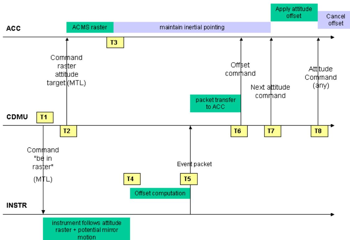
Figure 6 is illustrating the flow of information during a peak-up procedure.
