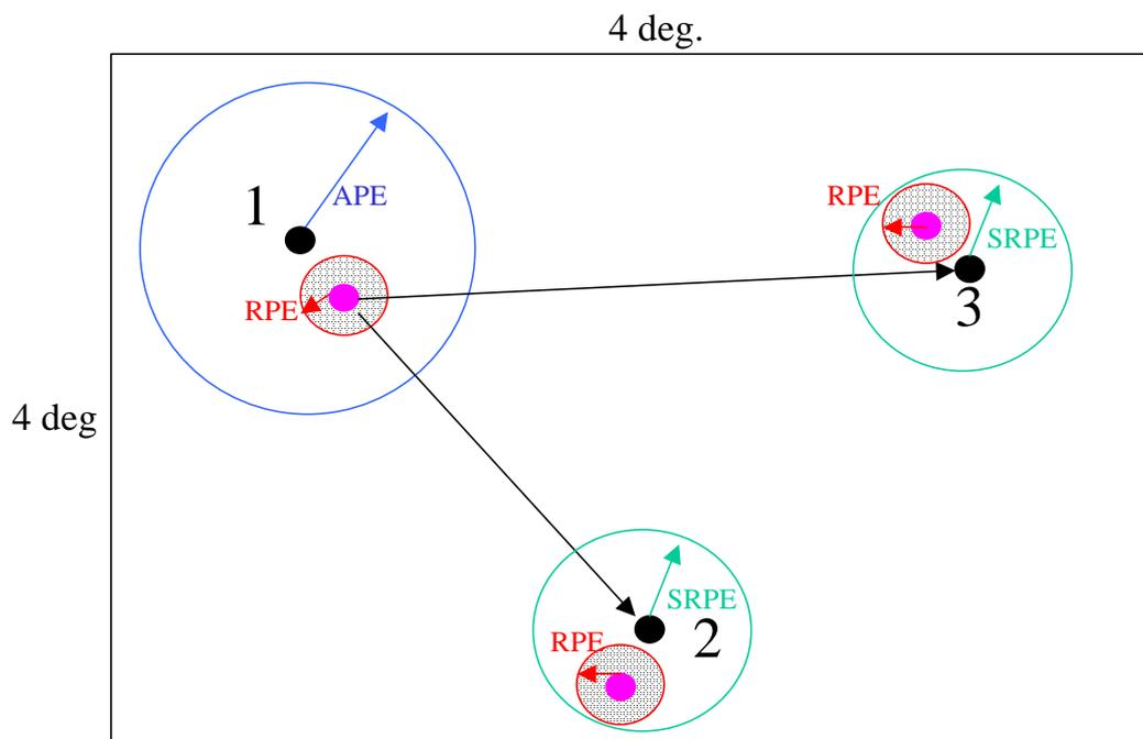
**Figure 1: Illustration of SRPE and its definition. The initial commanded direction (black dot no 1) is achieved within the APE accuracy (blue circle). The actual pointing of the spacecraft (dotted area within red circle) has an average direction (purple dot). New directions are commanded (black dot 2+3) relative to initial actual direction (purple dot 1) and are met within the SRPE requirement.**
