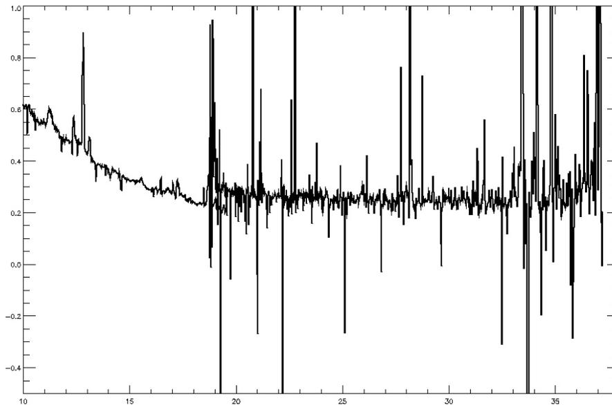
**Figure 3** SH and LH spectra of a stellar source, extracted in the standard pipeline. Noise in the LH spectrum is due to numerous outlying pixels within the 2-D extraction elements, not well treated by default dark current or pixel-pixel response calibrations.
