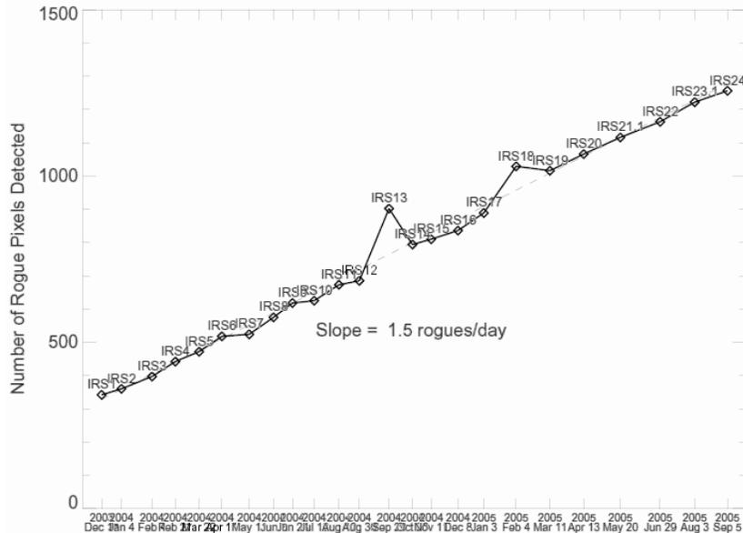
**Figure 2** Number of LH pixels exhibiting rogue behaviour since beginning of Routine Operations, demonstrating the accumulation of radiation damage since downward adjustment of the bias voltage near the end of the In-Orbit Checkout phase. [By J. Ingalls, from the SSC's public pages.]
