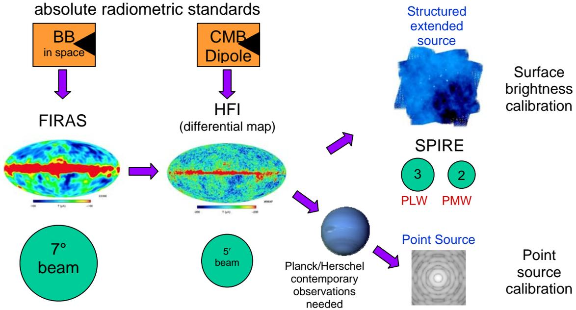
**Figure 2:** The traceability of HFI and SPIRE cross calibration to fundamental blackbody standards.
