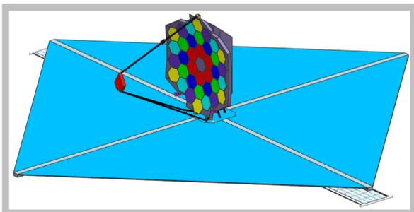
Right: Folded telescope in launch shroud. The spacecraft bus is below the telescope with the furled sunshield shown schematically by blue & pink bars; Above: deployed telescope with 20m-sized single-layer sunshield. The spacecraft bus is below the sunshield.
