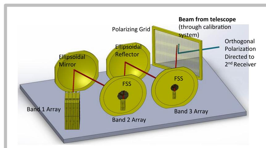
Above: Schematic of three-band receiver using two FSS for band separation. The concept can be extended to more bands as the highest-frequency band is dropped first, and thus suffers minimum loss.
