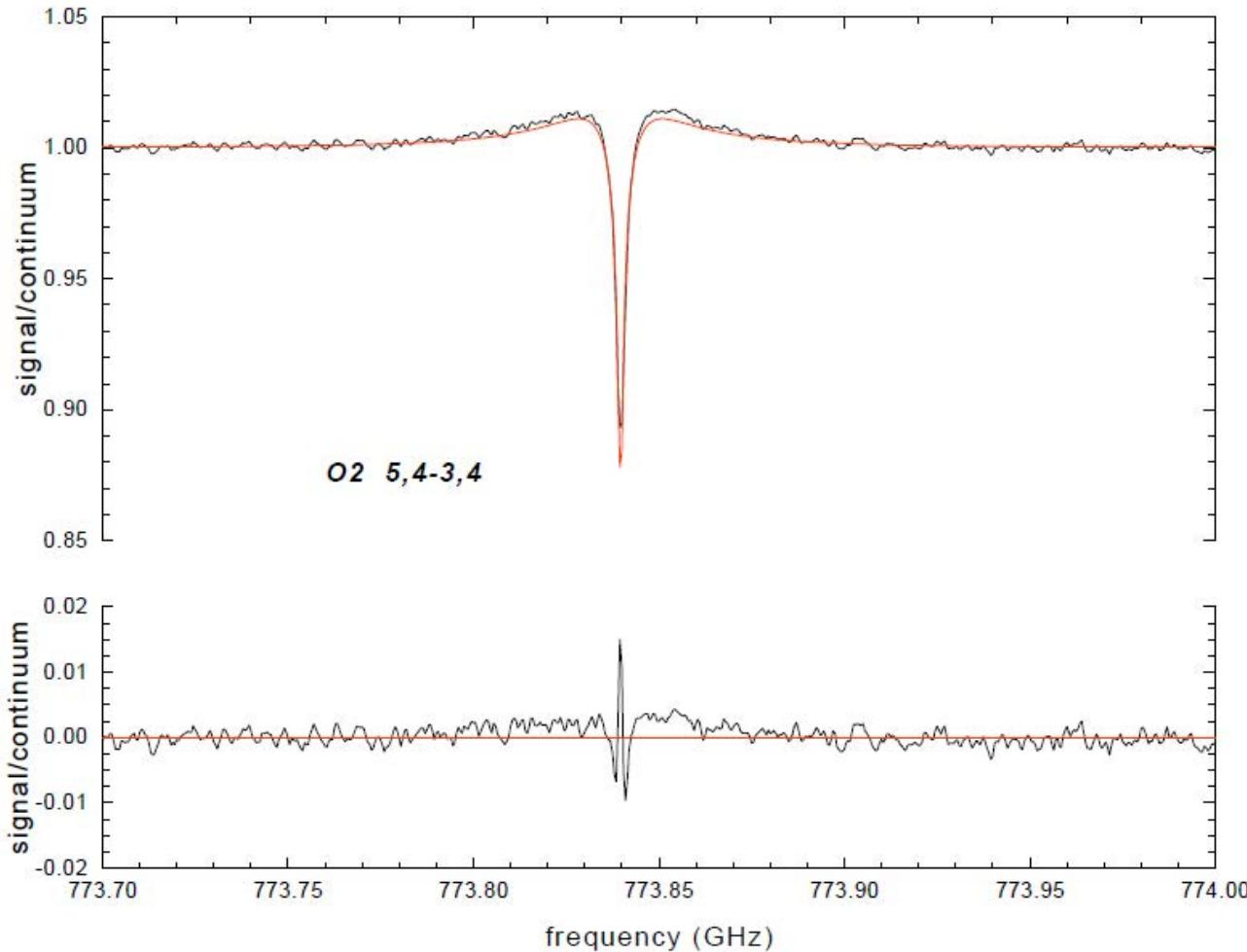
Fit of constant profile provides volume mixing ratio of 1400 ppm. However residual indicates that profile is not constant with altitude.
