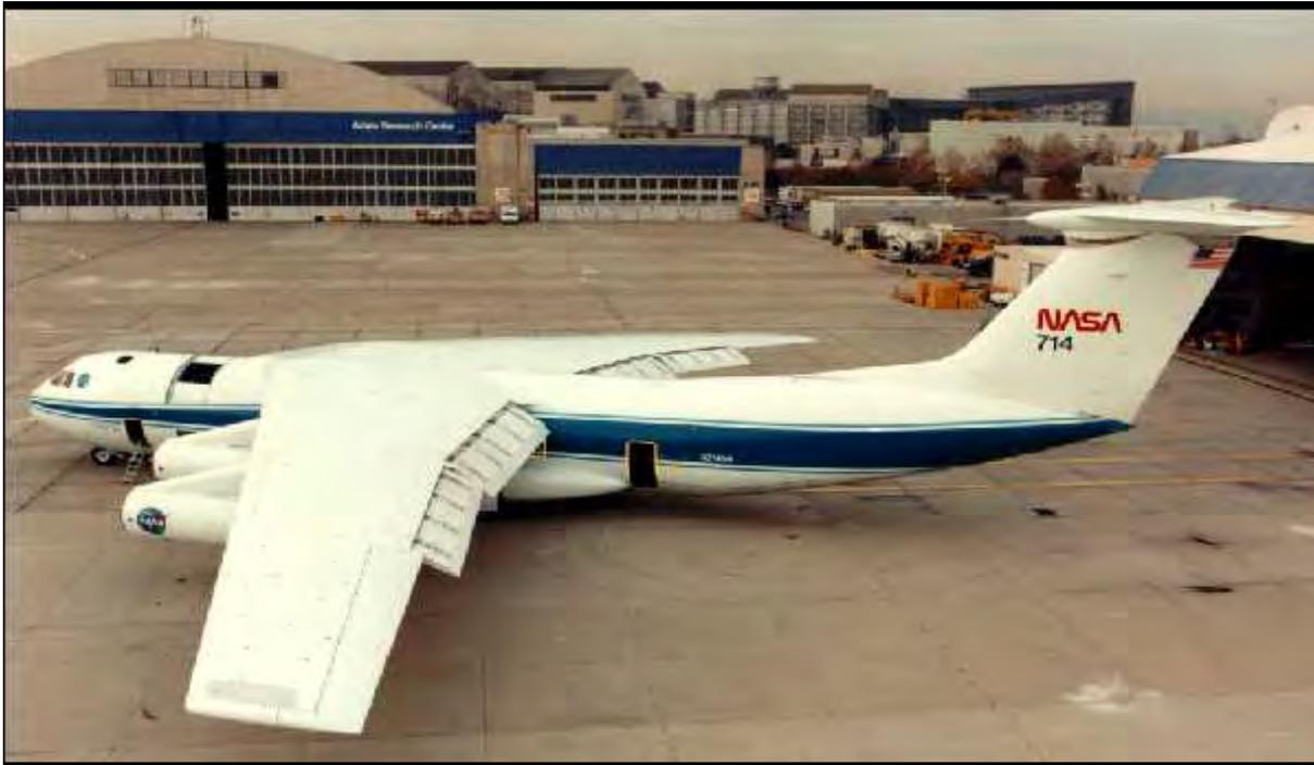
*NASA's Kuiper Airborne Observatory (KAO) C-141 with a 36-inch telescope onboard, based at NASA-Ames near San Francisco, flew from 1975 - 1996*
