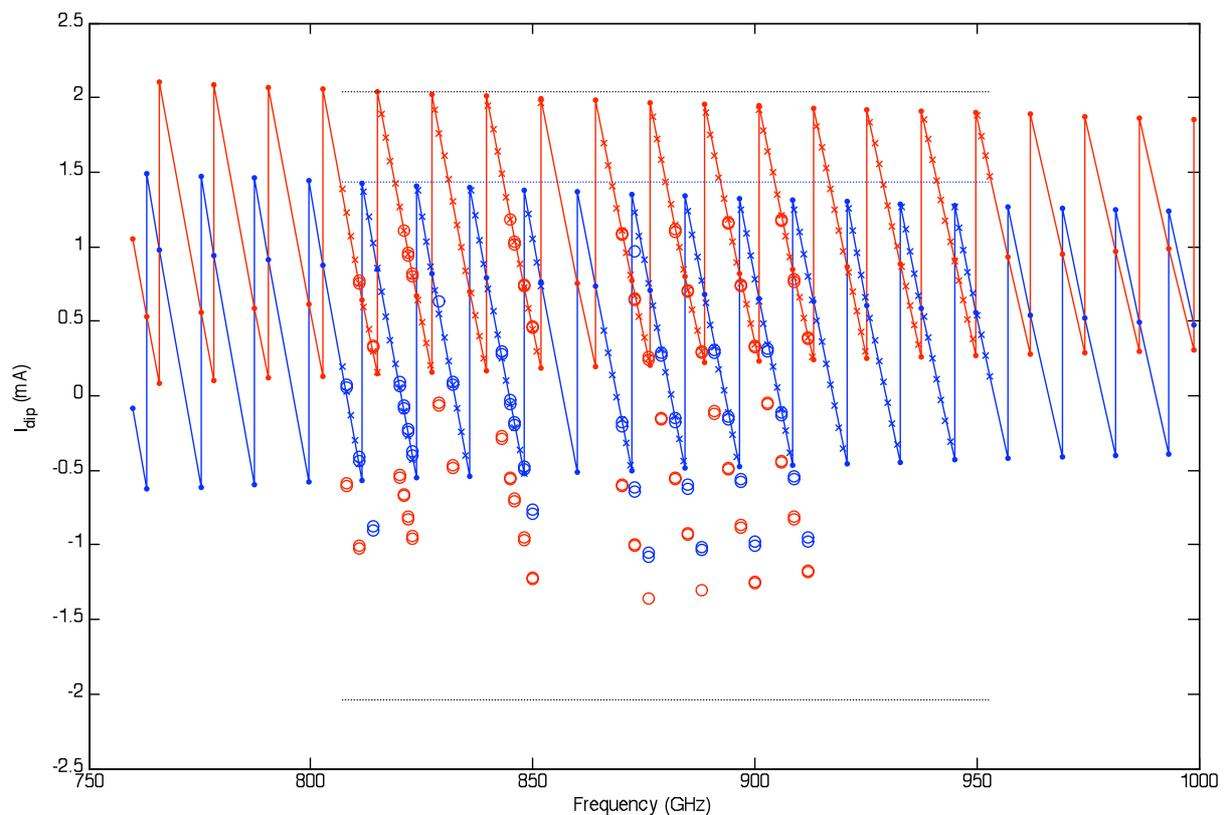
**Fig 3.-** LUT in band 3 together with clipping limits and measured data.
