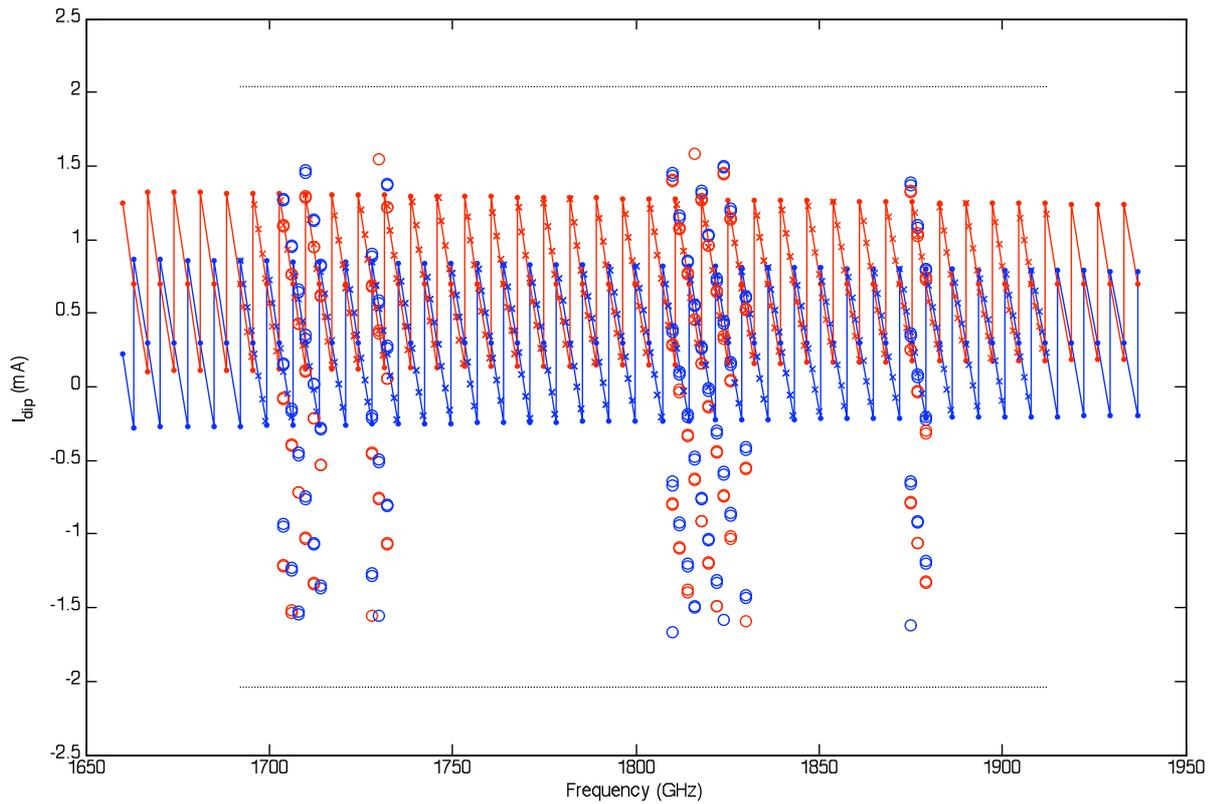
**Fig 6.-** LUT in band 7 together with clipping limits and measured data.
