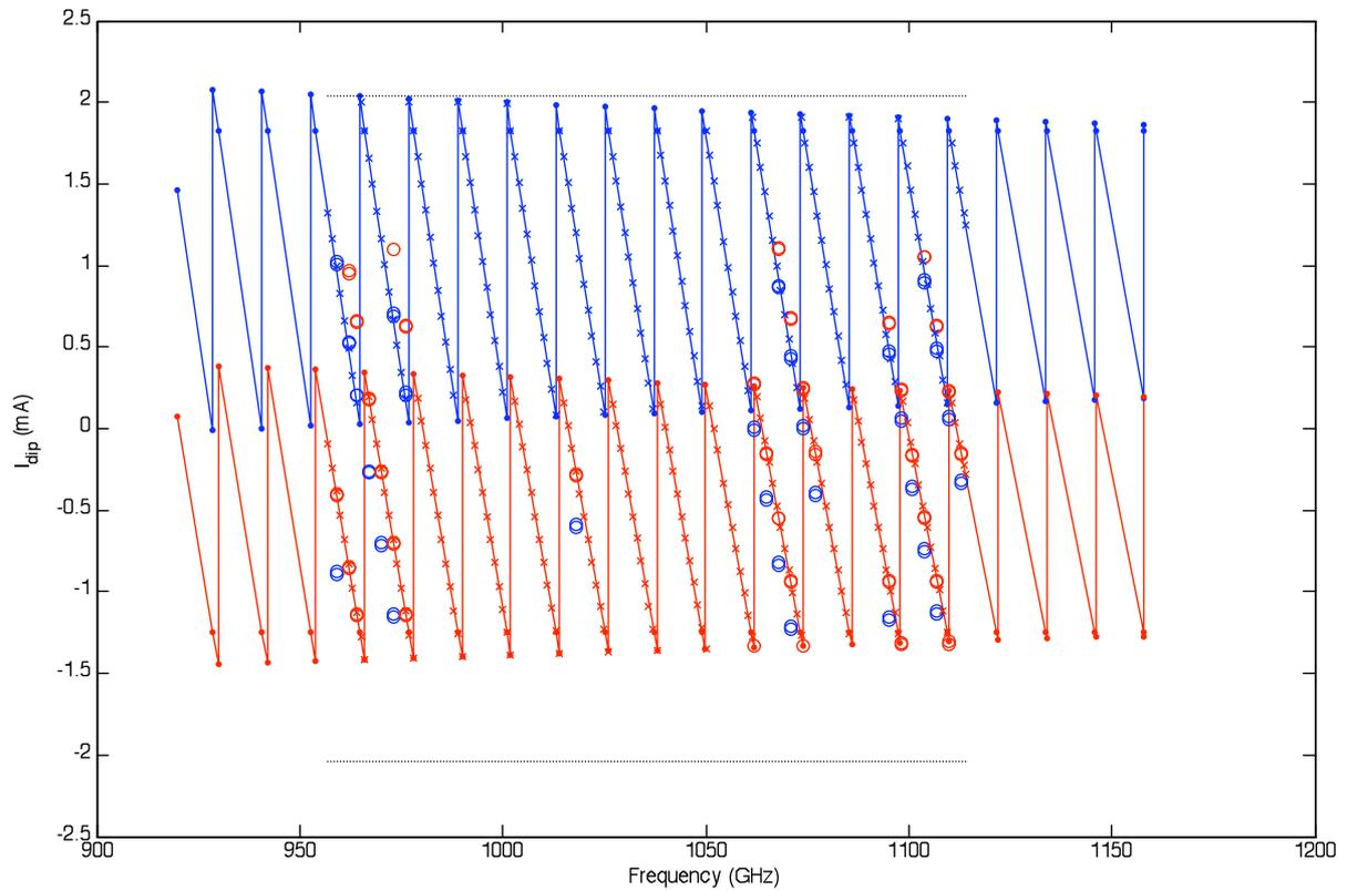
**Fig 4.-** LUT in band 4 together with clipping limits and measured data.
