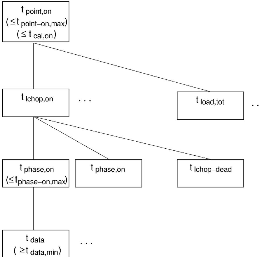
The number of  $t_{data}$  intervals within  $t_{phase,on}$  is given by  $n_{readout,on}$  which is  $\geq 1$ . The number of  $t_{ichop,on}$  intervals within  $t_{point,on}$  is given by  $(n_{load,on} + 1)n_{ichop-on,series}$  and the number of  $t_{load,tot}$  intervals within  $t_{point,on}$  by  $n_{load,on}$  where  $n_{ichop-on,series} \geq 1$  and  $n_{load,on} \geq 0$ .
