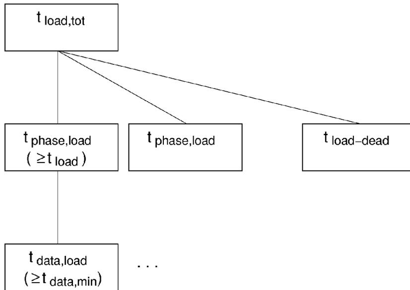
The load observation consists of two phases with equal length and a dead time. Each phase may contain several data readout intervals. Periods which may occur multiple times, but where the number of repetitions depends on the details of the observation are visualised by three dots here. The number of  $t_{data,load}$  intervals within  $t_{phase,load}$  is given by  $n_{readout,load}$  which is at least 1 and in most cases will be just 1.
