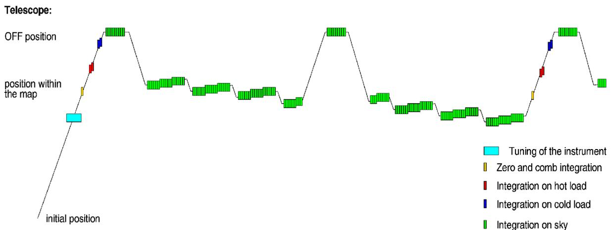
In case of different instrumental settings compared to the previous measurement a retuning of the instrument has to be performed as initial step. The actual observation always starts with a load calibration measurement (see Sect. 2.3), the main part of which can be performed during the initial slew to the OFF position. The OFF integration consists of a number of separate data dumps at the same position.
