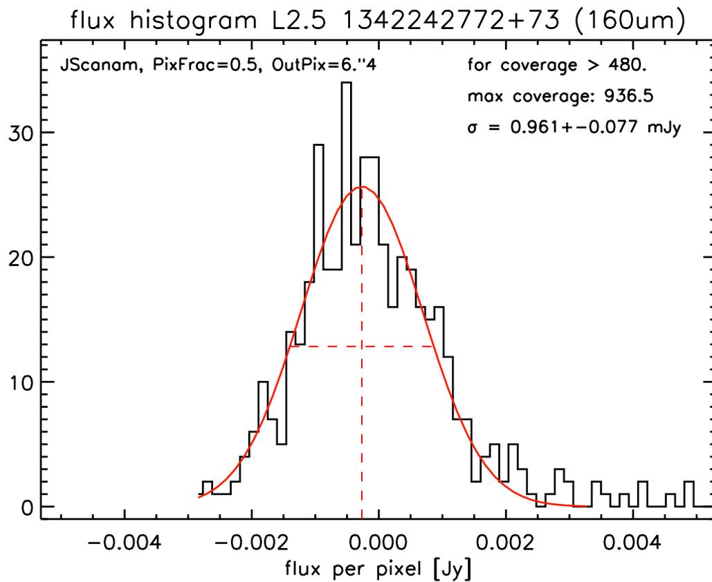
Figure 58: Noise determination for the 160  $\mu\text{m}$  coadded L2.5 map of OBSIDs 1342242772+73 with the histogram method (only the flux distribution around the background level is shown). The red curve represents the Gauss fit. The vertical red dashed line indicates the position of the average background level. The horizontal red dotted line indicates the FWHM ( $= 2\sqrt{2\ln 2}\sigma_{\text{hist}}$ ).
