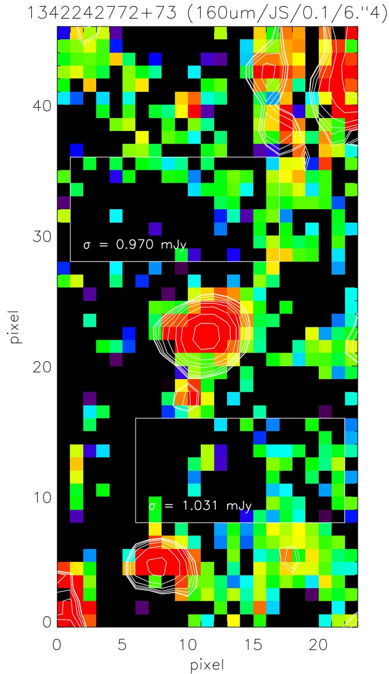
Figure 51: 160  $\mu\text{m}$  L2.5 combined JScanam map for OBSIDs 1342242772+73 with pixfrac 0.1 and output pixel size of 6".4. The two background fields for noise determination are outlined by the white boxes and the respective  $\sigma$  is indicated.
