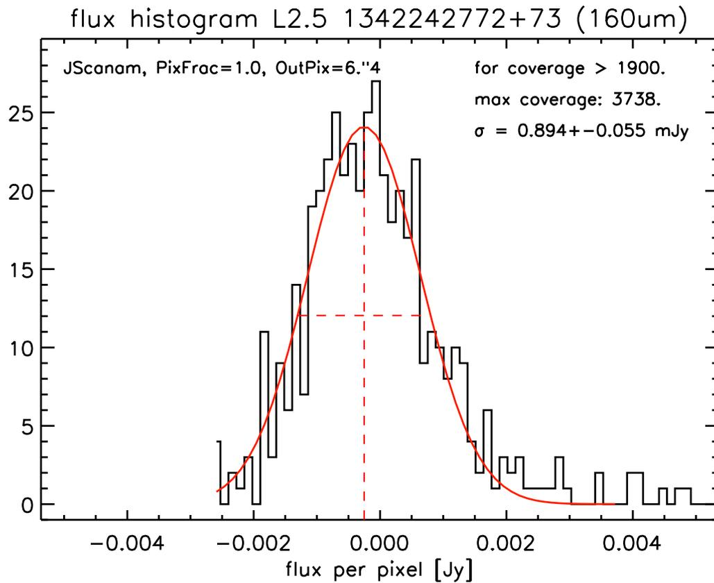
Figure 66: Noise determination for the 160  $\mu\text{m}$  coadded L2.5 map of OBSIDs 1342242772+73 with the histogram method (only the flux distribution around the background level is shown). The red curve represents the Gauss fit. The vertical red dashed line indicates the position of the average background level. The horizontal red dotted line indicates the FWHM ( $= 2\sqrt{2\ln 2}\sigma_{\text{hist}}$ ).
