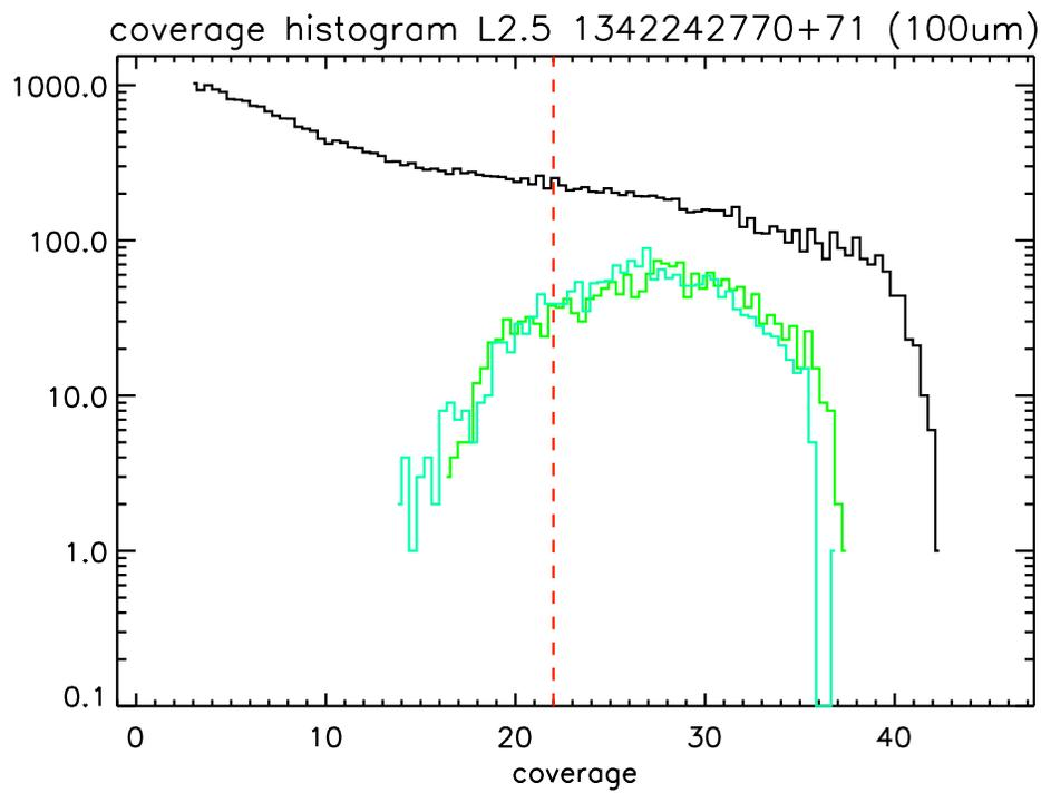
Figure 68: Histogram of the distribution of coverage for the L2.5 product with the SPG mapping parameter combination 15 / 0.1 / 1"6 (black, all values below a coverage value of 3.0 are cut). The red dashed line indicates the coverage threshold used in the noise analysis. The dark and light green histograms give the coverage distribution inside the source-free noise measurement areas 1 and 2, respectively. The corresponding image map is shown in Fig. 25.
