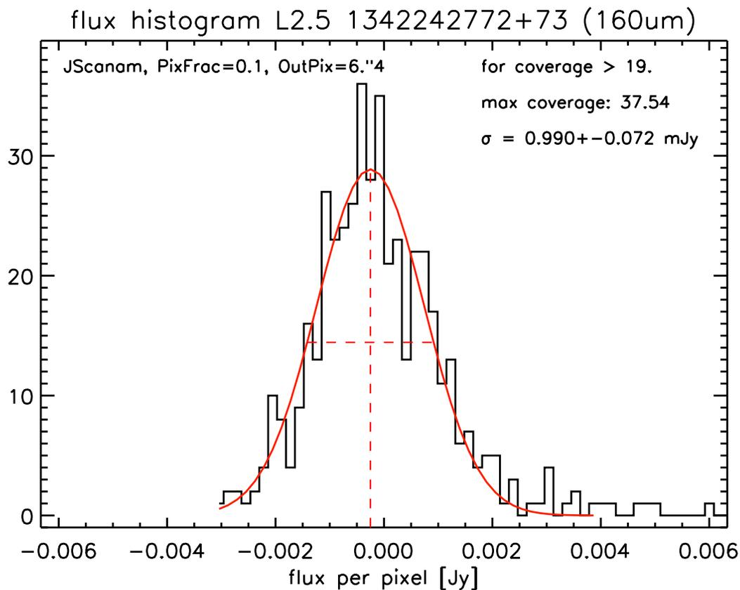
Figure 52: Noise determination for the 160  $\mu\text{m}$  coadded L2.5 map of OBSIDs 1342242772+73 with the histogram method (only the flux distribution around the background level is shown). The red curve represents the Gauss fit. The vertical red dashed line indicates the position of the average background level. The horizontal red dotted line indicates the FWHM ( $= 2\sqrt{2\ln 2} \sigma_{\text{hist}}$ ).
