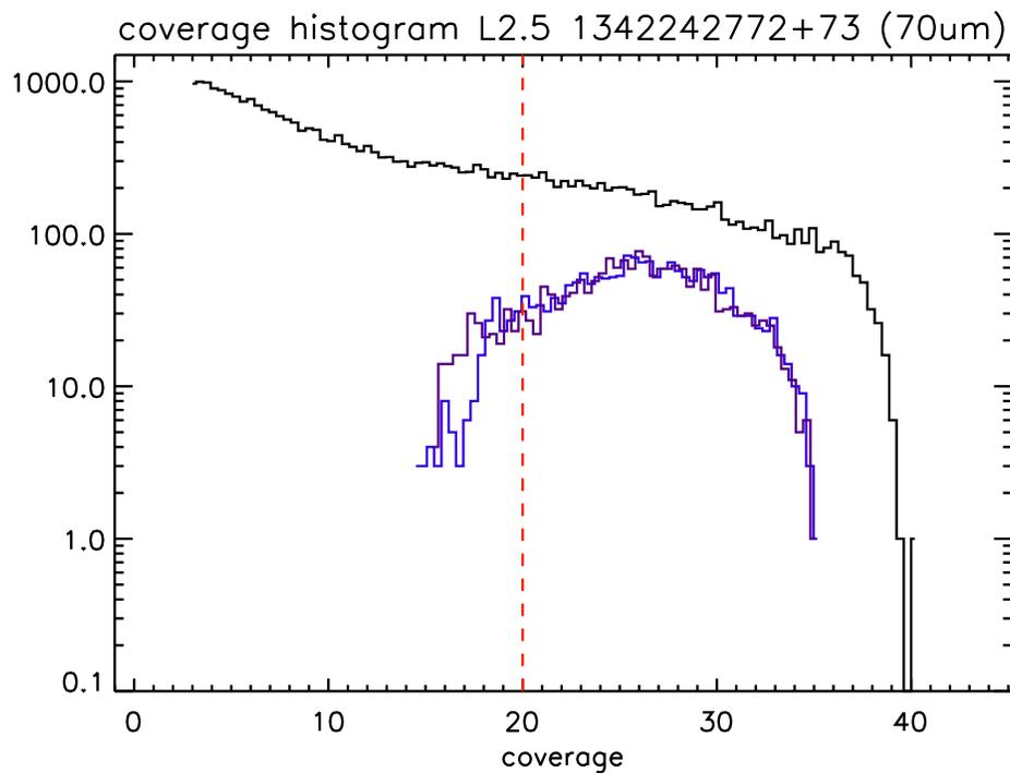
Figure 67: Histogram of the distribution of coverage for the L2.5 product with the SPG mapping parameter combination 15 / 0.1 / 1"6 (black, all values below a coverage value of 3.0 are cut). The red dashed line indicates the coverage threshold used in the noise analysis. The dark blue and violet histograms give the coverage distribution inside the source-free noise measurement areas 1 and 2, respectively. The corresponding image map is shown in Fig. 3.
