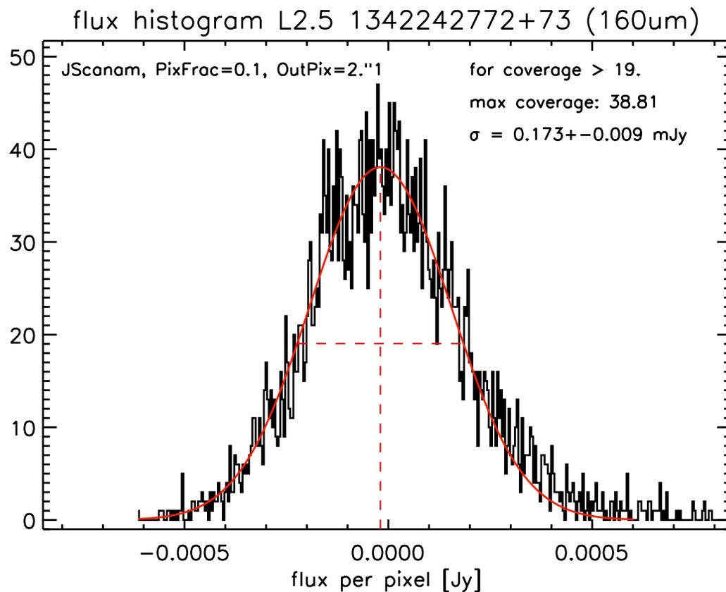
Figure 46: Noise determination for the 160  $\mu\text{m}$  coadded L2.5 map of OBSIDs 1342242772+73 with the histogram method (only the flux distribution around the background level is shown). The red curve represents the Gauss fit. The vertical red dashed line indicates the position of the average background level. The horizontal red dotted line indicates the FWHM ( $= 2\sqrt{2\ln 2}\sigma_{\text{hist}}$ ).
