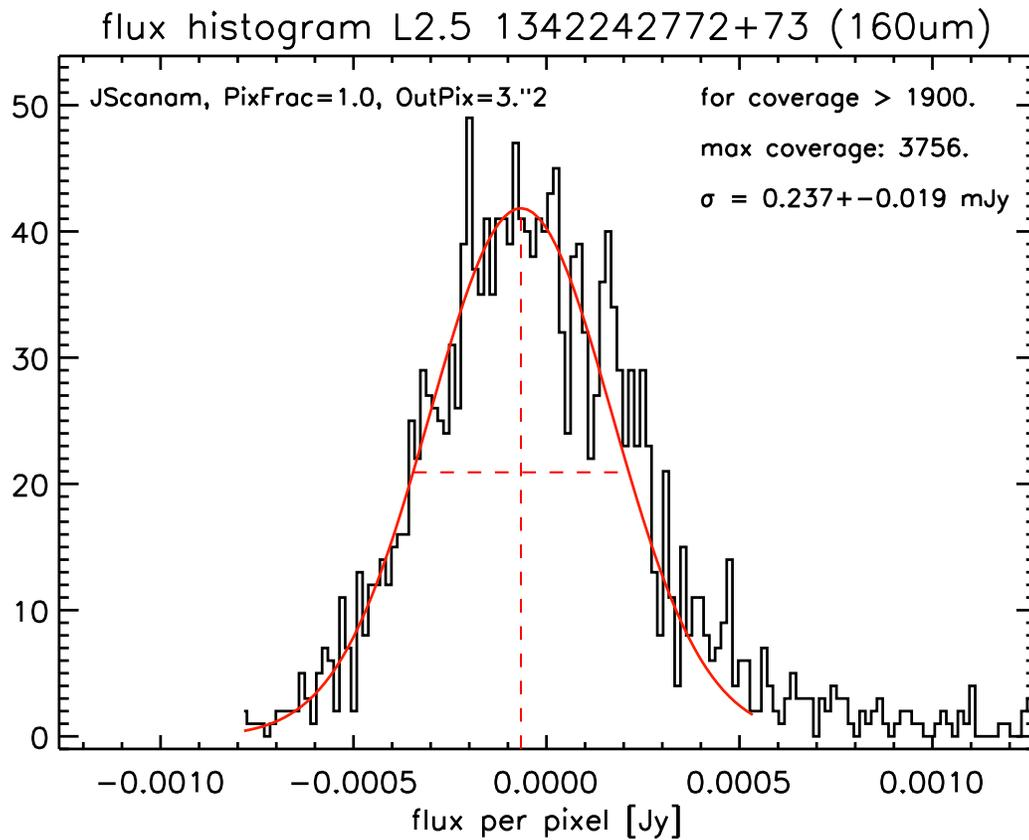
Figure 62: Noise determination for the 160  $\mu\text{m}$  coadded L2.5 map of OBSIDs 1342242772+73 with the histogram method (only the flux distribution around the background level is shown). The red curve represents the Gauss fit. The vertical red dashed line indicates the position of the average background level. The horizontal red dotted line indicates the FWHM ( $= 2\sqrt{2\ln 2}\sigma_{\text{hist}}$ ).
