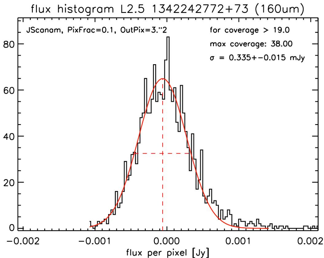
Figure 48: Noise determination for the 160  $\mu\text{m}$  coadded L2.5 map of OBSIDs 1342242772+73 with the histogram method (only the flux distribution around the background level is shown). The red curve represents the Gauss fit. The vertical red dashed line indicates the position of the average background level. The horizontal red dotted line indicates the FWHM ( $= 2\sqrt{2\ln 2}\sigma_{\text{hist}}$ ).
