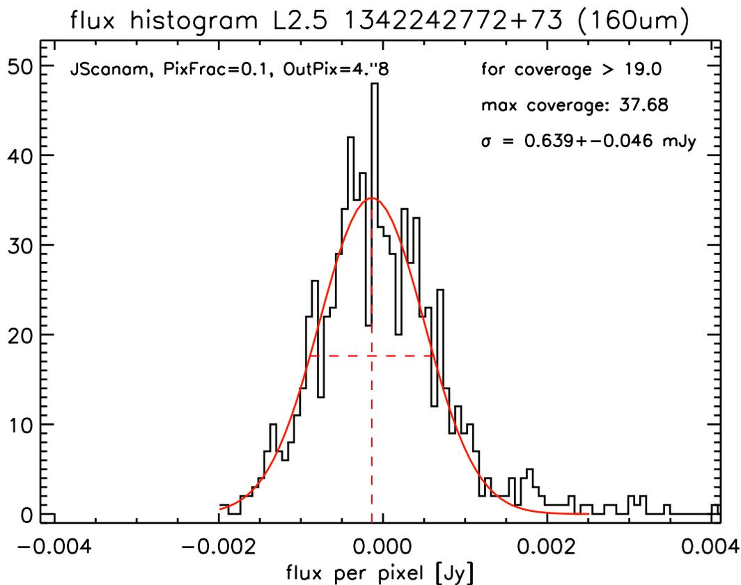
Figure 50: Noise determination for the 160  $\mu\text{m}$  coadded L2.5 map of OBSIDs 1342242772+73 with the histogram method (only the flux distribution around the background level is shown). The red curve represents the Gauss fit. The vertical red dashed line indicates the position of the average background level. The horizontal red dotted line indicates the FWHM ( $= 2\sqrt{2\ln 2}\sigma_{\text{hist}}$ ).
