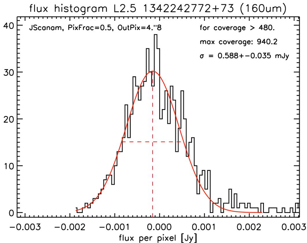
Figure 56: Noise determination for the 160  $\mu\text{m}$  coadded L2.5 map of OBSIDs 1342242772+73 with the histogram method (only the flux distribution around the background level is shown). The red curve represents the Gauss fit. The vertical red dashed line indicates the position of the average background level. The horizontal red dotted line indicates the FWHM ( $= 2\sqrt{2\ln 2}\sigma_{\text{hist}}$ ).
