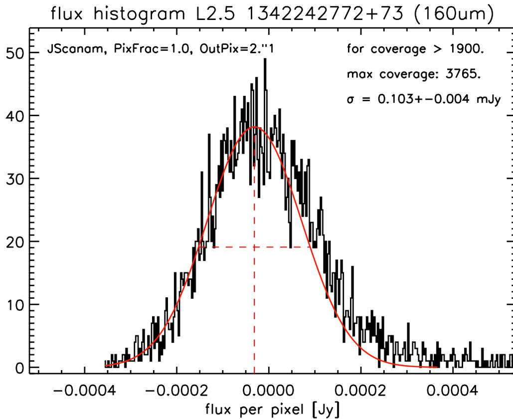
Figure 60: Noise determination for the 160  $\mu\text{m}$  coadded L2.5 map of OBSIDs 1342242772+73 with the histogram method (only the flux distribution around the background level is shown). The red curve represents the Gauss fit. The vertical red dashed line indicates the position of the average background level. The horizontal red dotted line indicates the FWHM ( $= 2\sqrt{2\ln 2}\sigma_{\text{hist}}$ ).
