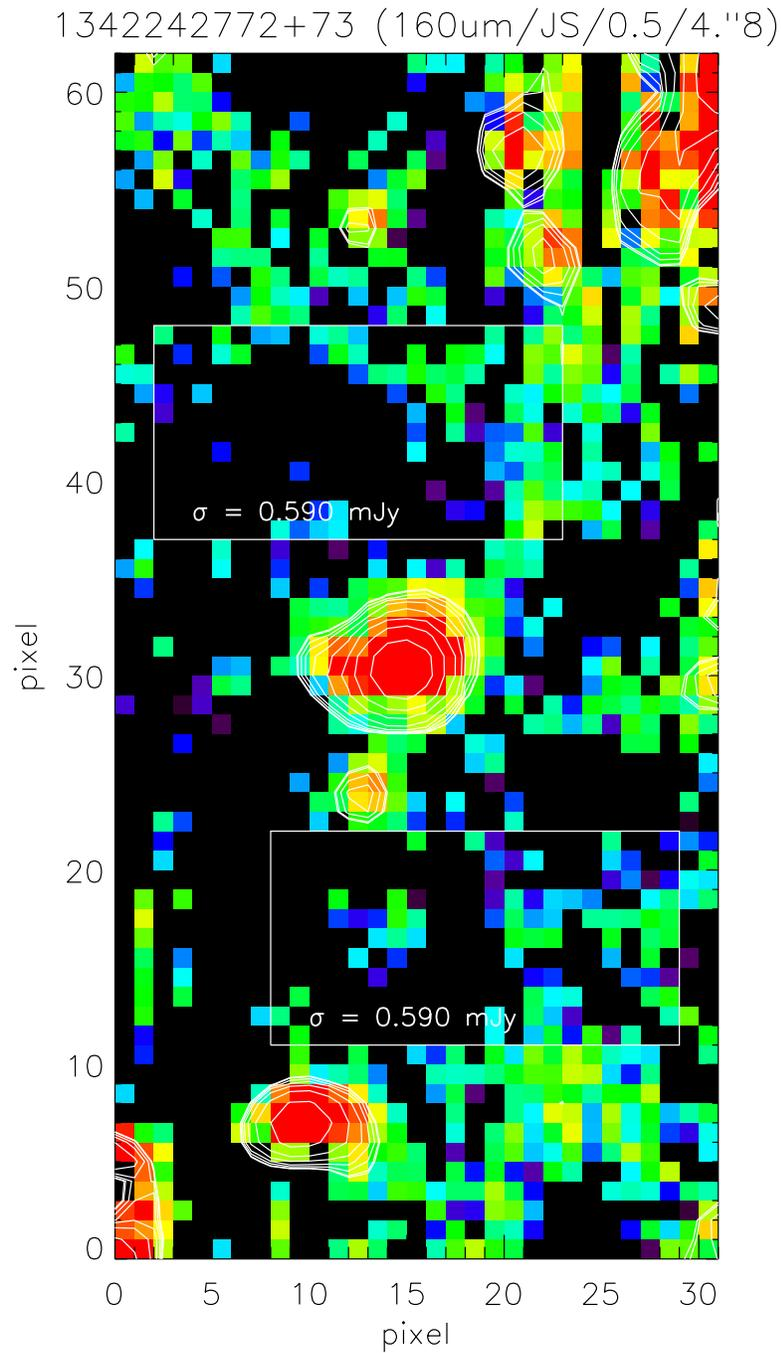
Figure 55: 160  $\mu\text{m}$  L2.5 combined JScanam map for OBSIDs 1342242772+73 with pixfrac 0.5 and output pixel size of 4".8. The two background fields for noise determination are outlined by the white boxes and the respective  $\sigma$  is indicated.
