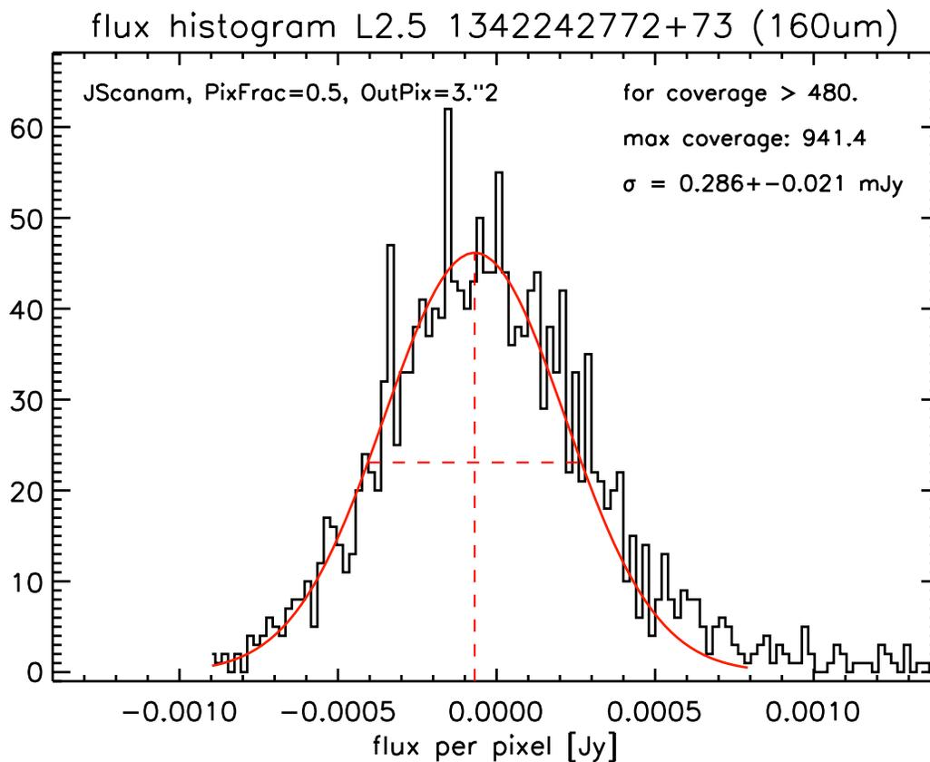
Figure 54: Noise determination for the 160  $\mu\text{m}$  coadded L2.5 map of OBSIDs 1342242772+73 with the histogram method (only the flux distribution around the background level is shown). The red curve represents the Gauss fit. The vertical red dashed line indicates the position of the average background level. The horizontal red dotted line indicates the FWHM ( $= 2\sqrt{2\ln 2}\sigma_{\text{hist}}$ ).
