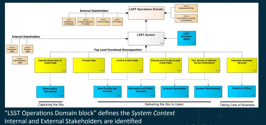
Decomposition of system into 6 Top Level Functions (yellow)
