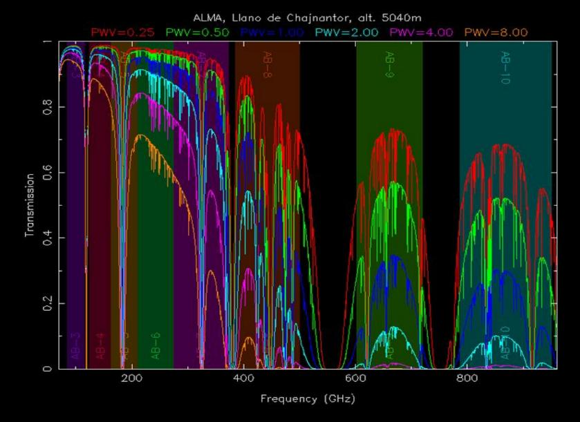
The exceptionally low water vapor content of Chajnantor gives access to submillimeter windows down to ~300 microns
