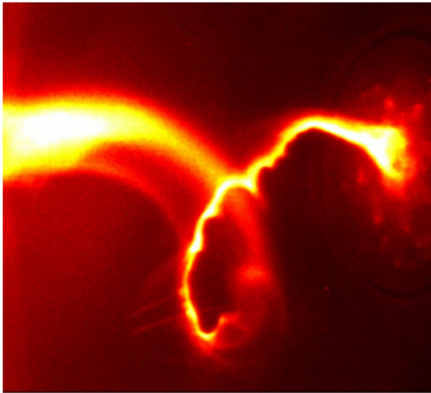
An argon plasma jet forms a rapidly growing corkscrew, known as a kink instability. This instability causes an even faster-developing behavior called a Rayleigh-Taylor instability, in which ripples grow and tear the jet apart. This phenomenon, the Caltech researchers say, has never been seen before and could be important in understanding solar flares and in developing nuclear fusion as a future energy source. Watch the plasma in action [here](#).
