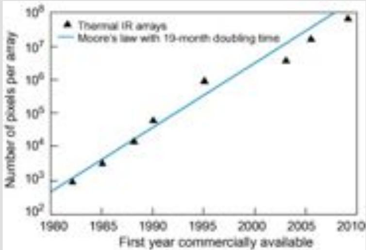
Advances in IR detectors impelled the development of wide-field instruments shaping our view of the cold Universe.
