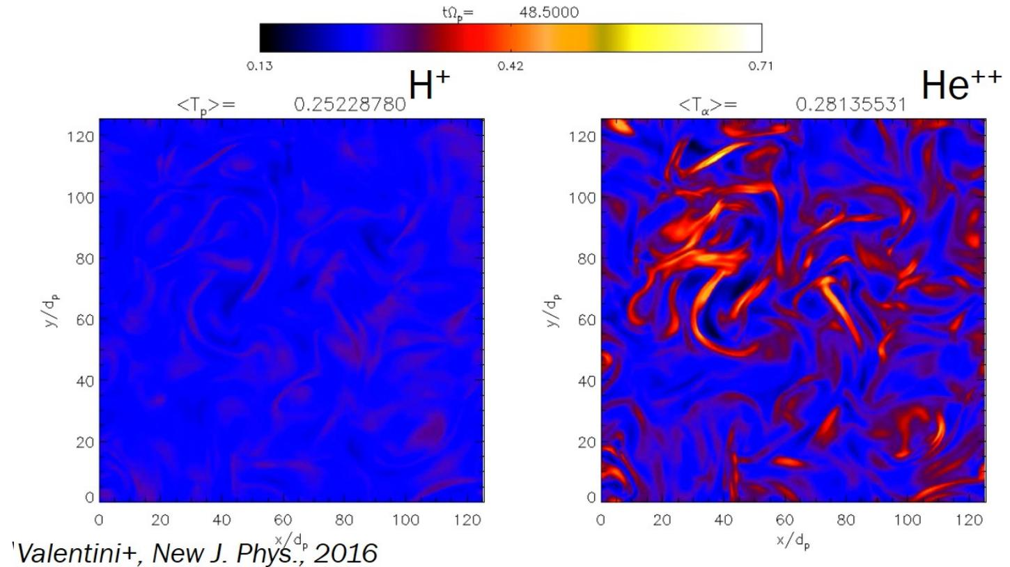
Necessary to quantify the **energy partition among protons and alphas** at kinetic scales.
