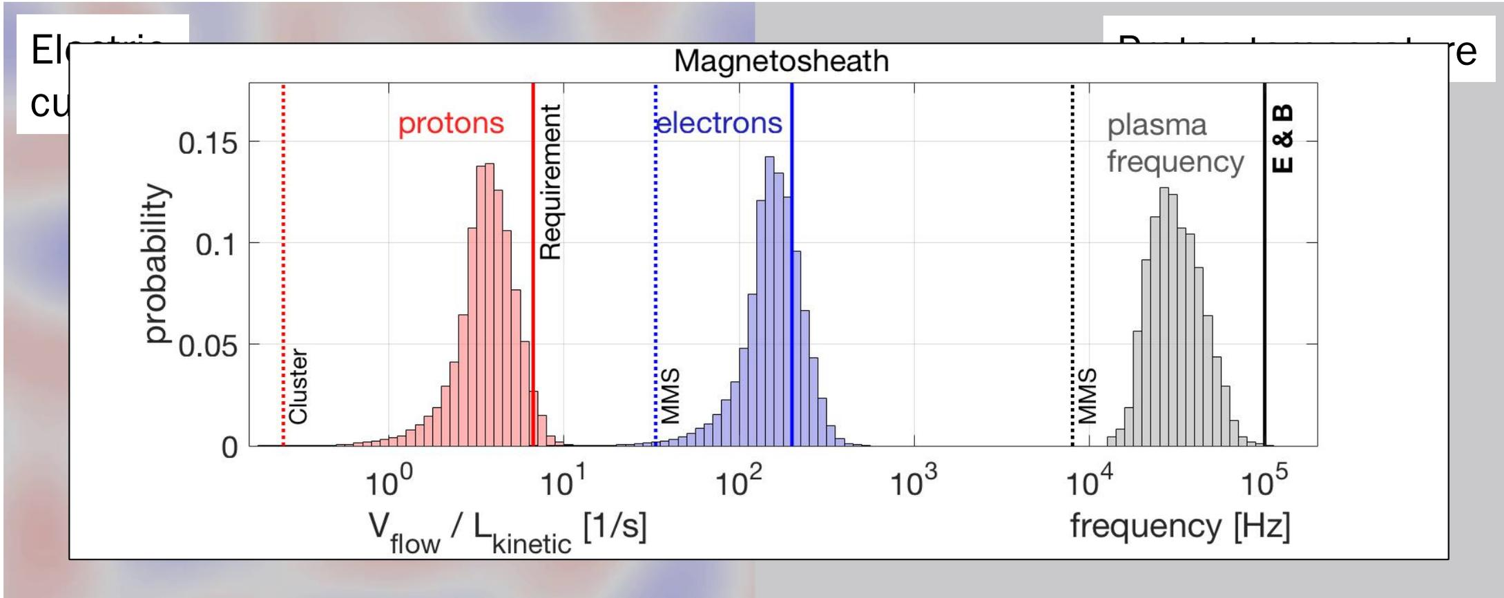
**THOR shall resolve:** plasma distribution functions at kinetic scales of electrons and mass-resolved ions, 3D electric and magnetic fields at plasma frequency.
