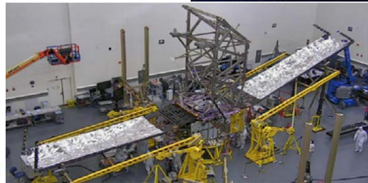
Forward Sunshield Unitized Pallet Structure Attached to the Spacecraft Bus (Northrop Grumman)
