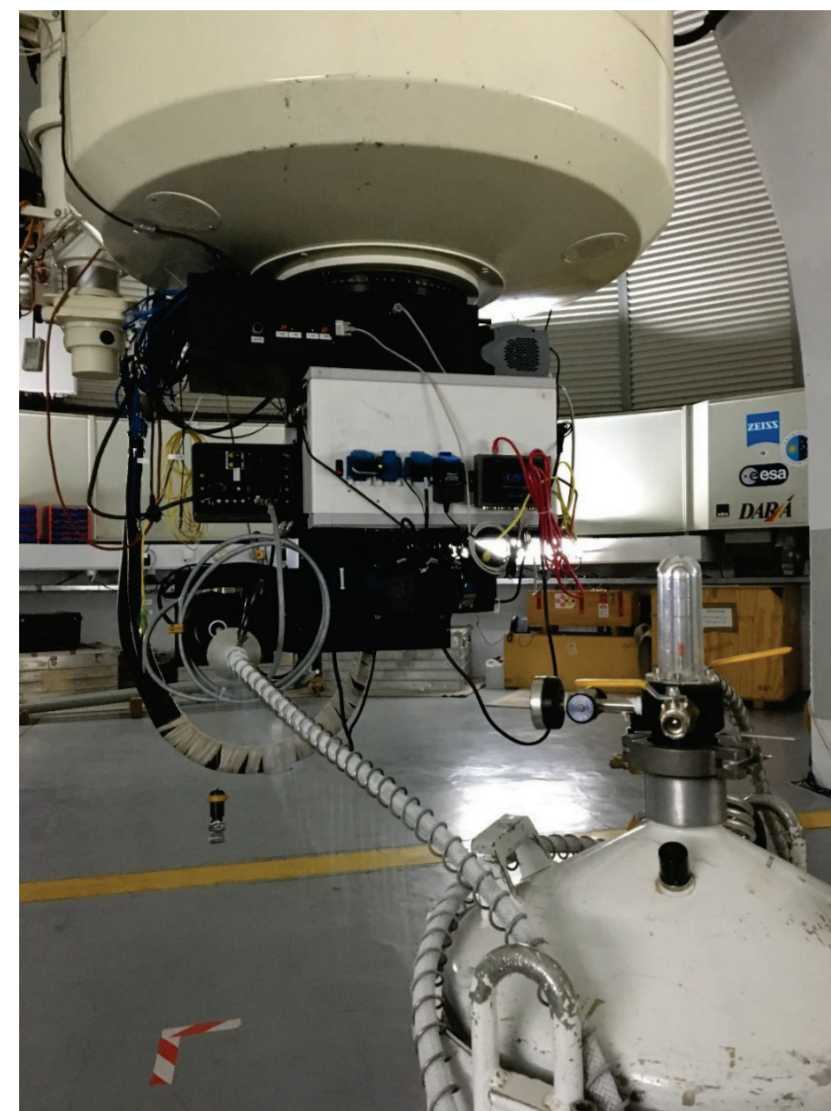
Figure 1: View of the Spectrograph mounted on the OGS telescope, while being filled with liquid nitrogen. The detector array is operated at -100\text{ }^{\circ}\text{C} .
