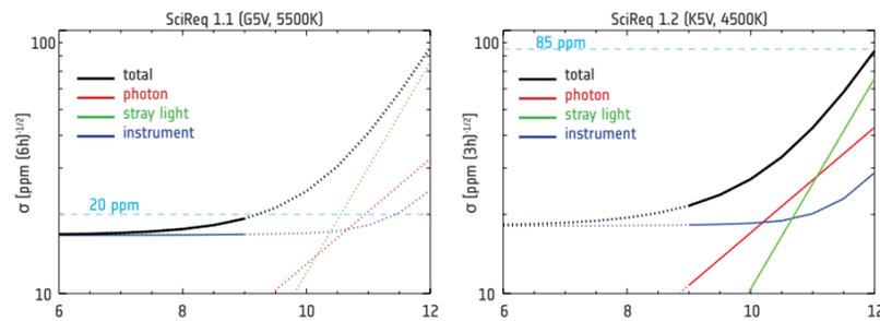
1-sigma photometric precision (in parts per million) for two sizing cases. **Left:** precision foreseen after a total on-source integration time of 6 hours (duration of transit of planet with orbital period of 50 days). **Right:** precision foreseen after a total on-source integration time of 3 hours (duration of transit of planet with orbital period of 13 days). The dashed horizontal lines denote requirements.
