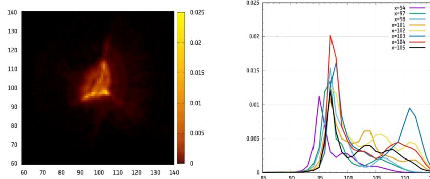
Left: White light PSF measured over 500 - 800 nm waveband during the on-ground calibration campaign (x- and y-axes in pixels relative to bottom lower left pixel in a 200x200 pixel image frame, colour scale indicates fraction of total power in an individual pixel); Right: Cuts through the PSF at the specified value of x. Credit: University of Bern.
