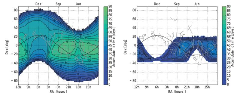
Accessible sky (in days per year) for which the contribution to the noise budget from Earth stray light is  $\leq 5 \text{ ppm} / 70 \text{ ppm}$  for a  $V=9$  G-type ( $T_{\text{eff}}=5500\text{K}$ ) /  $V=12$  K-type ( $T_{\text{eff}}=4500\text{K}$ ) dwarf, and for which the maximum % of each spacecraft orbit that is free from interruptions due to Earth Occultation or passage through the South Atlantic Anomaly is 50% (**left**) or 80% (**right**). Solid black line: locus of the Sun.
