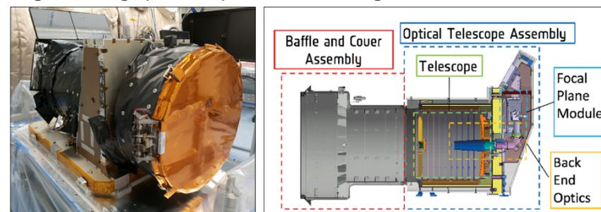
Left: Fully-assembled flight model of the CHEOPS payload; Right: Cross-section through the payload. Credit: University of Bern.
