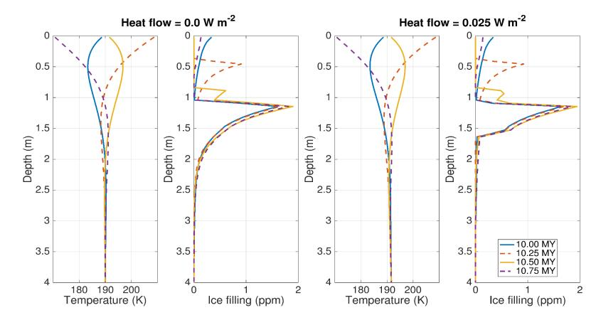
Subsurface temperatures and fraction of ice in pore space after 10 Martian years, calculated with a heat flow of 0.0 W/m<sup>2</sup> (left) and 0.025 W/m<sup>2</sup> (right).
