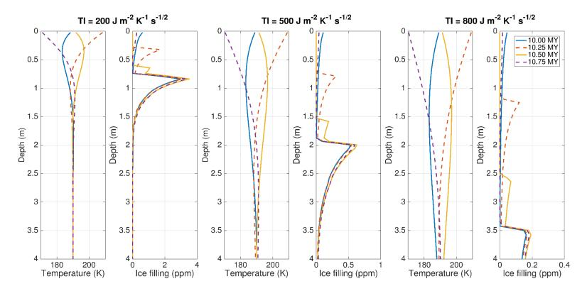
Subsurface temperatures and fraction of pore space filled with ice after 10 Martian years for different thermal inertias.
