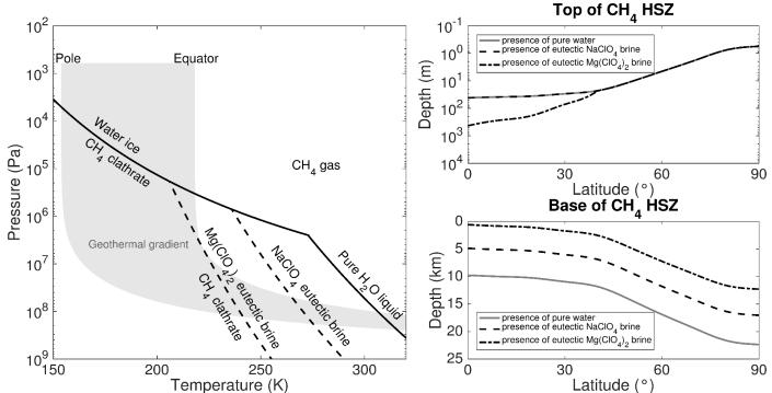
Mg(ClO<sub>4</sub>)<sub>2</sub> exhibits one of the lowest eutectic temperature of all salts (206K) and its presence, in addition to shift the base of HSZ, significantly affects the top of HSZ at low latitudes.
