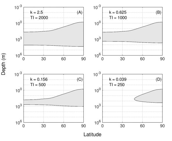
Stability zones are calculated using mean annual surface temperatures and assuming a surface heat flow of 19 mW m<sup>-2</sup>, the present-day average value (Parro et al., 2017).
