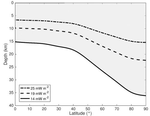
Variations in the depth of the base of methane hydrate stability zone as a function of latitude for different values of the heat flow (14, 19 and 25 mW  $m^{-2}$ ).
