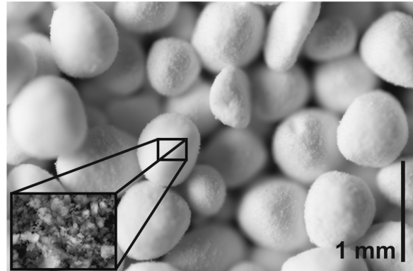
Fig. 1: Image of the mm-sized dust aggregates used in the experiments. The inset shows a SEM image of the micrometer-sized silica particles forming the aggregates.
