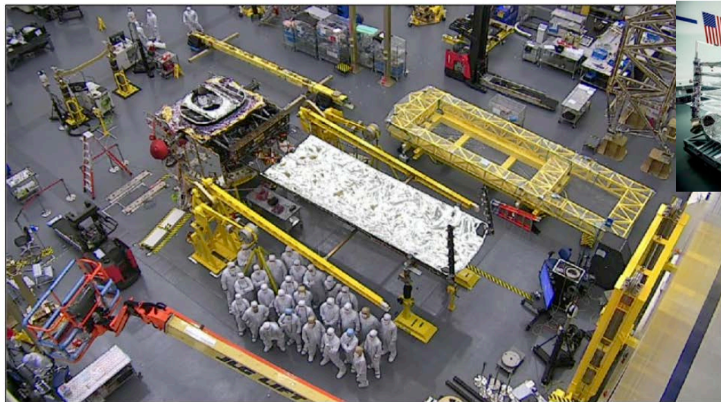
Forward Sunshield Unitized Pallet Structure Attached to the Spacecraft Bus (Northrop Grumman)
