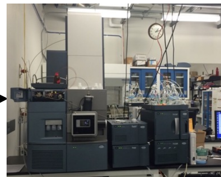
Liquid chromatography with fluorescence detection and time-of-flight mass spectrometry
