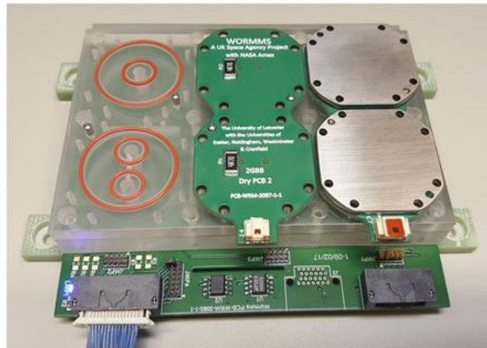
Figure 1. (A) Expanded computer-aided design illustration of the 'Deep Space Petri-Pod' (DSPP) design layers. (B) Photograph of the DSPP breadboard prototype, including electronic circuit board control system.
