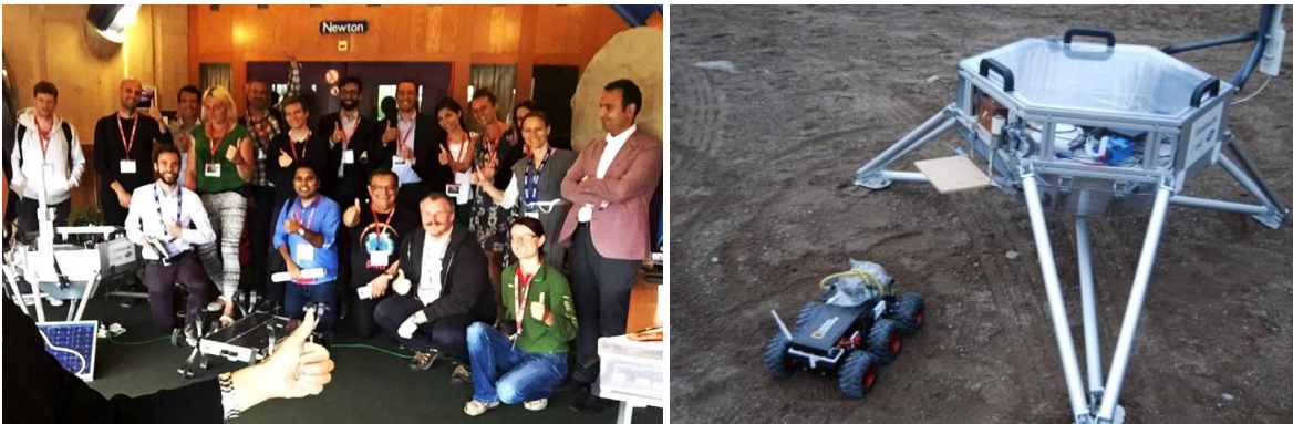
Fig 1 (left) : we thank ILEWG EuroMoonMars 2017 campaign crew at ESTEC (here with ExoGeoLab lander & Puli Rover) & at simulation campaigns (PMAS, LUNEX1, IcAres) at LunAres base, Poland. Fig. 2 (right), ILEWG ExoGeoLab lander with remotely controlled USB4000 spectrometer and rover
