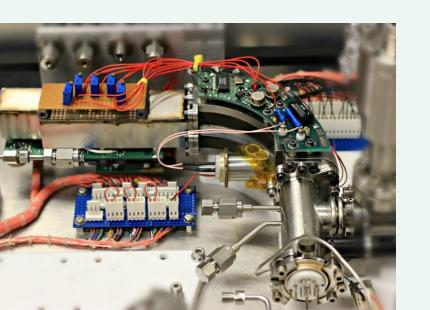
6 cm radius 90° magnetic sector MS • Triple collectors for CNO isotopes • Dual collector for D/H • SEM for noble gases • m/z range 2-150 amu
