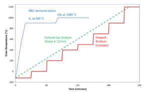
Figure 2: Example sample oven heating profiles
