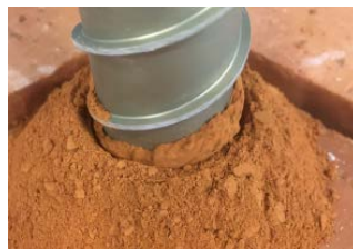
Figure 1: ProSEED drill – electrode coverage example
