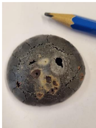
Figure 1: Crystalline synthetic analog sample of High-Mg Region major-element composition.
