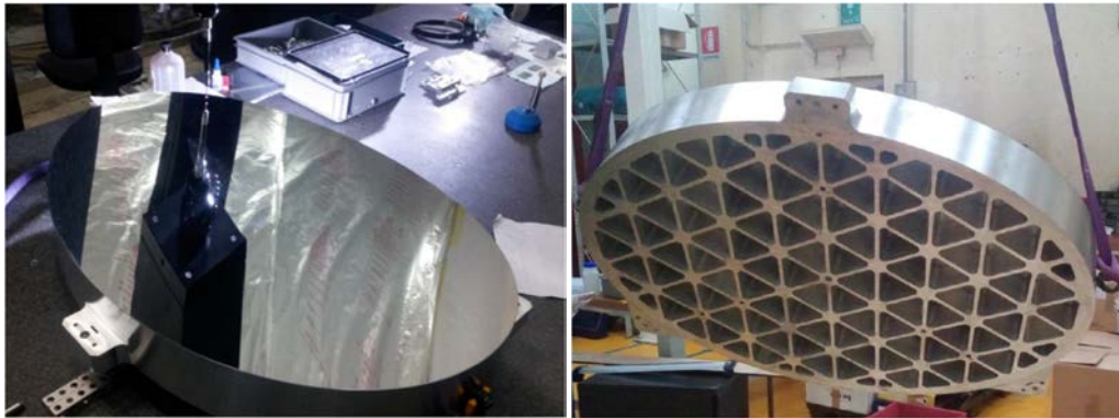
Figure 4-11: PTM mirror after milling and diamond turning processes completed including undergoing CMM measurement of surface form (left)
