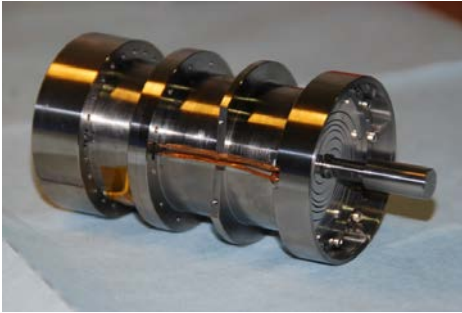
Figure 4-7: (Upper left) Cooler system parameter sizing; (Lower left) 2K cooler motor mechanism (mass is 820g); (Right) JT Cooler Schematic.
