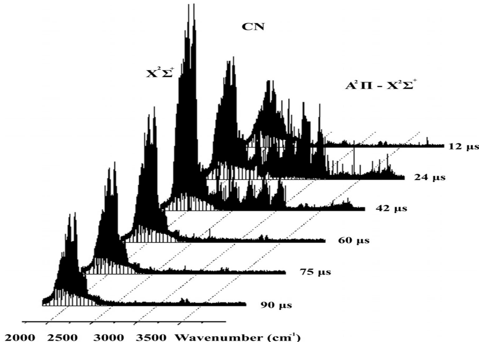
The time-resolved emission FT spectrum from a pulsed discharge in a (CN)<sub>2</sub> and He mixture. The discharge pulse duration was 20μs. The 30 time-resolved spectra were collected from t = 0–90 μs with a step of 3 μs. The spectra of C<sub>2</sub>H<sub>2</sub> and C<sub>2</sub> were observed at 3300 and 3600 cm<sup>-1</sup>.
