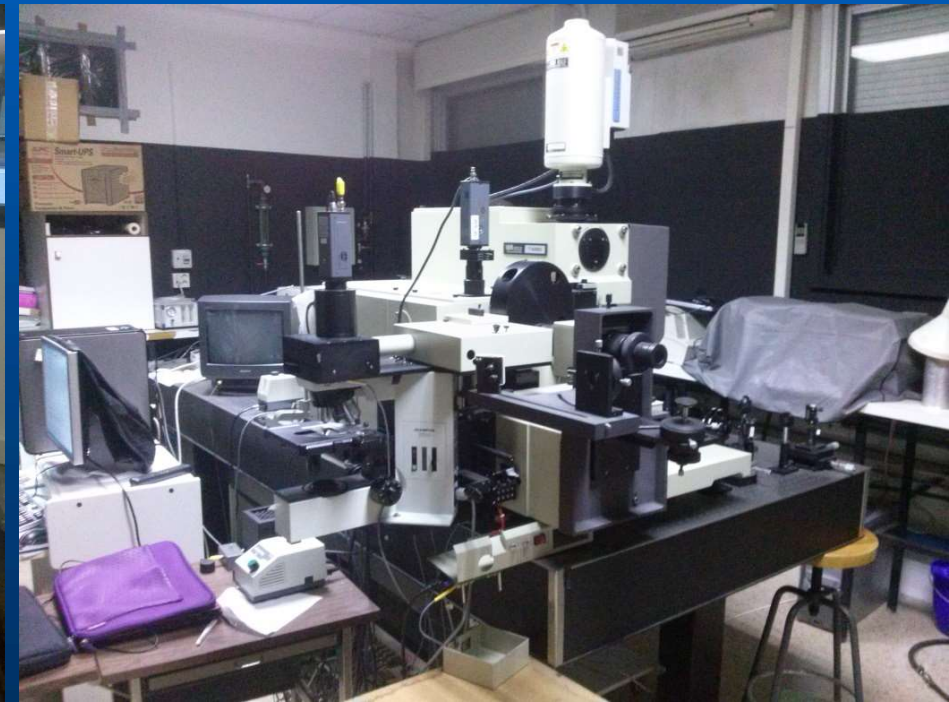
Ar-ion laser with a Jobin-Yvon T-6400 Raman spectrometer of 1 \mu\text{m} res.) at ICMAB-CSIC
