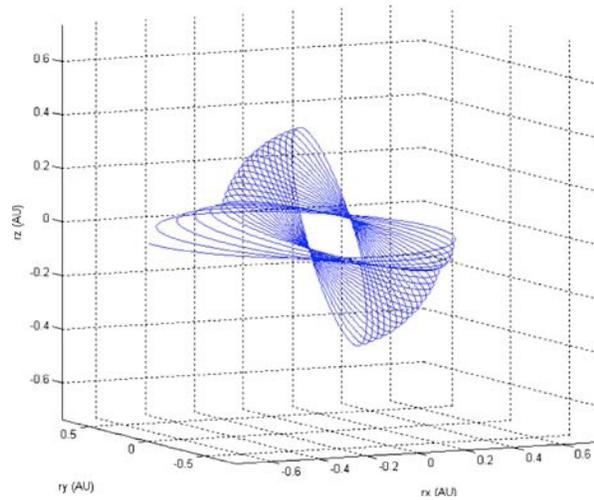
*Figure 7: The orbital scenario for the POLARIS proposal (Appourchaux et al. 2009) using a VGA and a sail of side dimension 179 m.*
