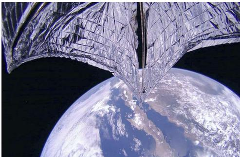
Whereas the solar sail option does not require carrying a large mass of propellant, it does require storage and deployment of a solar sail over two orders of magnitude larger than any previously flown.
