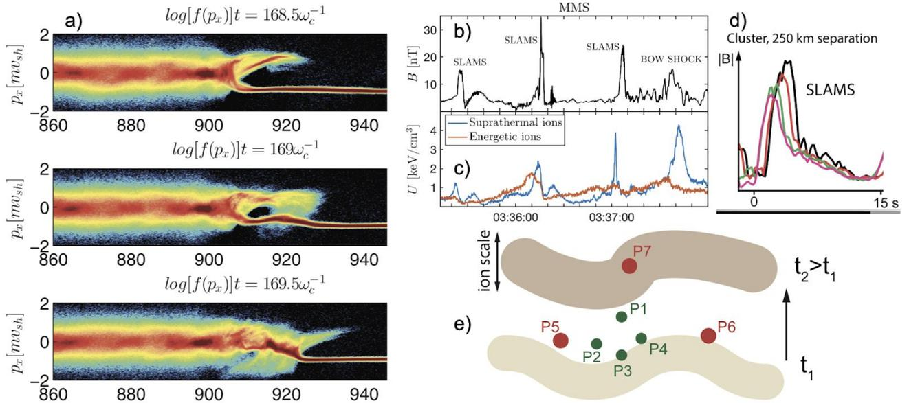
Figure 3. *Quasi-parallel shock. a) Kinetic simulations of the time evolution of ion injection at a quasi parallel shock with Mach number  $M=20$  (Caprioli+, ApJL, 2015). b-c) MMS measurements of ion energization by SLAMS (Johlander+, 2019) d) SLAMS evolution in Cluster data (Lucek+, JGR, 2008), e) sketch illustrating the need of 7 spacecraft to resolve spatio-temporal variations at SLAMS.*
