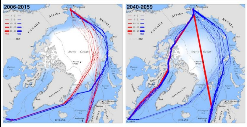
Red lines indicate fastest available routes for moderately ice-hardened vessels (PC6) Blue lines indicate fastest available routes for common open-water ships. Credit: L.C. Smith and S.R. Stephenson, PNAS.
